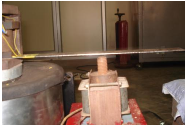
Plate 4.2 Magnetic shaker below the cantilever
