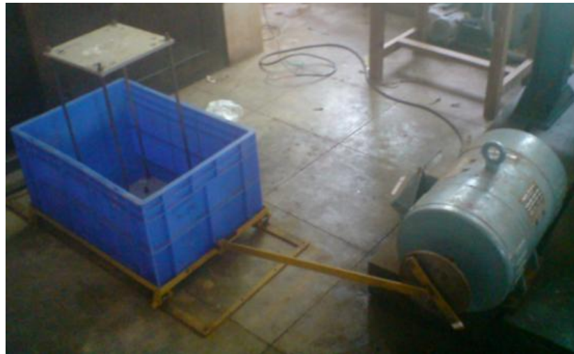
Plate 4.5 Experimental set up for simplified berthing structure model
