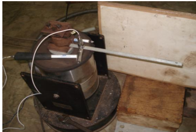
Plate 4.1 Cantilever fixed on shaker
