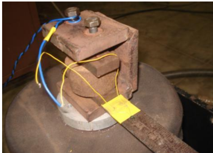
Plate 4.7 Strain gauge connected to experimental setup
