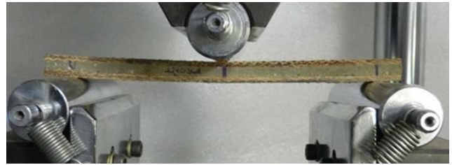
FIG. 3. Sandwich sample mounted on flexural test set-up [Color figure can be viewed in the online issue, which is available at wileyonlinelibrary.com].
