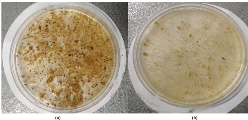
Fig. 5 Aerobic sludge granulation of a dicamba treatment reactor and b control reactor
