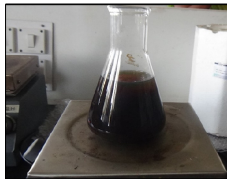
Fig. 4. Upgrading of CTPO by mechanically stirring a suspension of silica gel in diluted CTPO.
