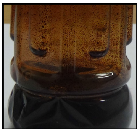
Fig. 10. Gummy deposits formed during storage of CTPO.
