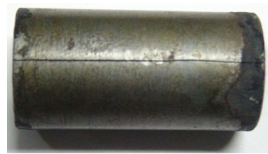
Fig. 4 Crack propagation in EN31 steel probe quenched in water
