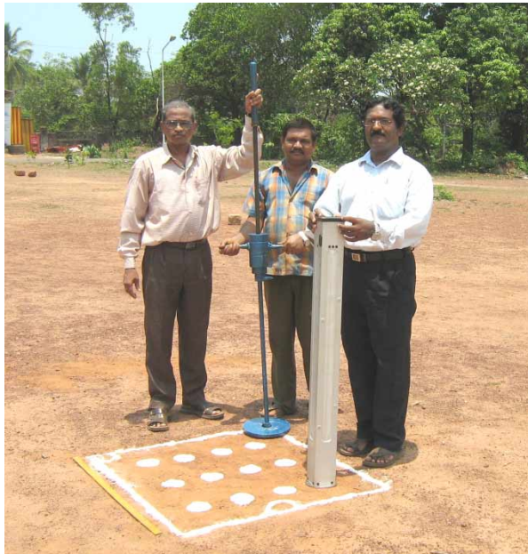
Figure 8. Deployment of PFWD and DCP at site.
