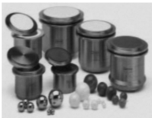
Fig. 2. Grinding jars and balls.
