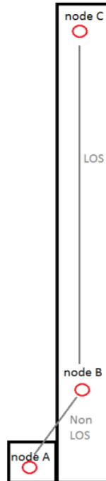
Figure 8. Example of using dual hops from Node A to Node B to Node C.
