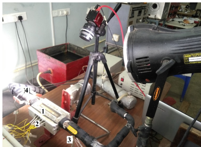
Fig. 3 Rear view of the experimental setup: (1) Rectangular aluminum block consisting of two rectangular channels, (2) Thermocouples to measure wall temperature, (3) Thermocouple to measure channel inlet temperature, and (4) Thermocouple to measure outlet fluid temperature
