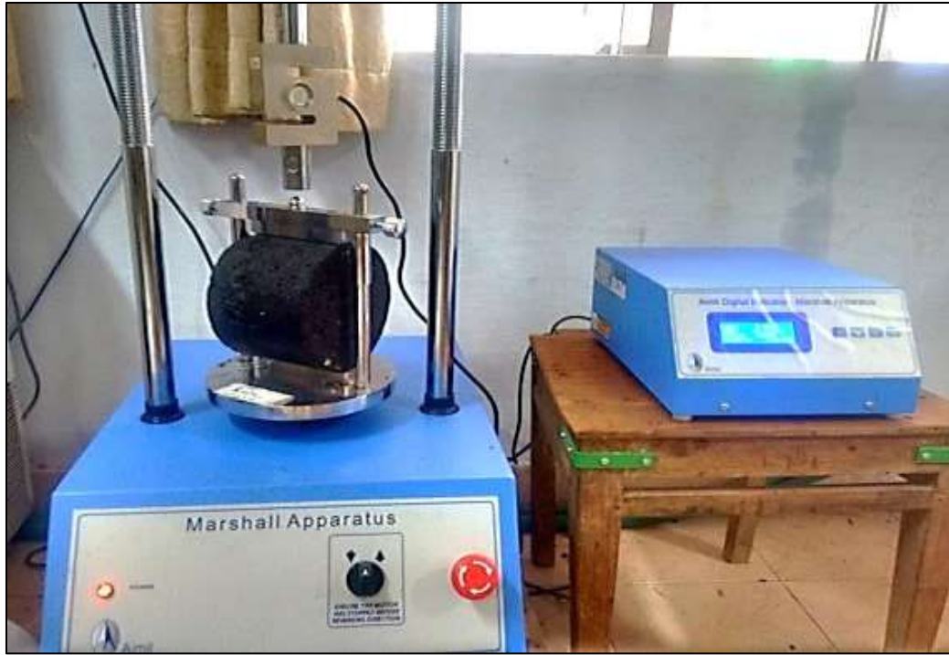
Fig. 3.5. Indirect tensile strength test setup
