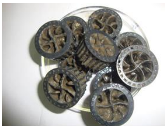
Figure 3.3 Biofilm growth upon the surface of the carrier media.
