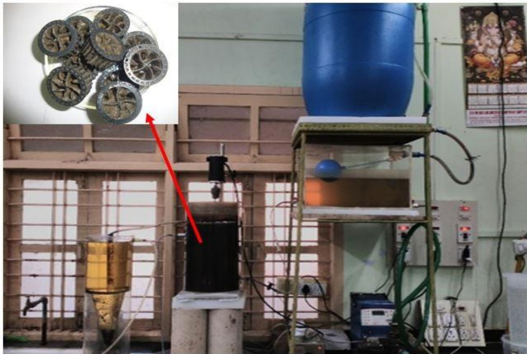
Figure 3.1 Lab scale AS-biofilm reactor for Phase 1 studies
