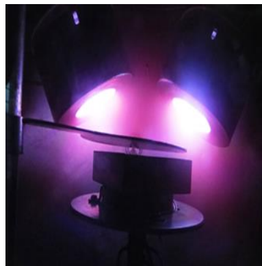
Figure 2.5 Plasma during sputtering process.
