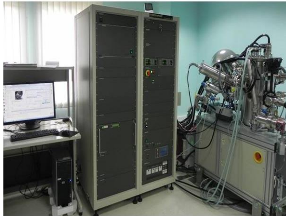
Figure 2.25 X-ray Photoelectron Spectrometer (Model: PHI 5000 Versaprobe II, FEI Inc.) (Image source: https://www.iitk.ac.in/acms/spectroscopylab.html ).
