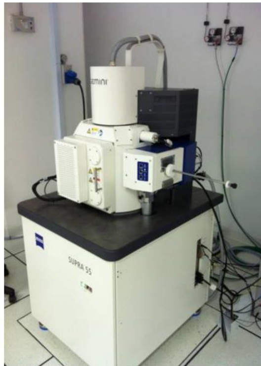
Figure 2.11 Field Emission Scanning Electron Microscope (Model: SUPRA 55, CARL ZEISS-GERMANY). (Imagesource: http://www.mse.ntu.edu.sg/Research/create/Documents/Equipment%20Details-FESEM%20Supra%2055.pdf )
