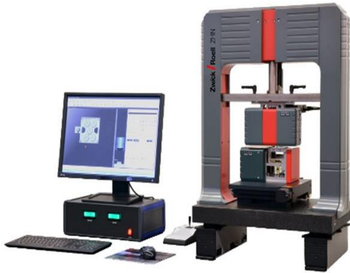
Figure 2.21 Nanoindenter (ASMEC Universal nanomechanical Tester (ZHN)). (Imagesource: https://www.zwick.com/en/hardness-testers-for-instrumented-indentation-tests/zhn-nanoindenter ).
