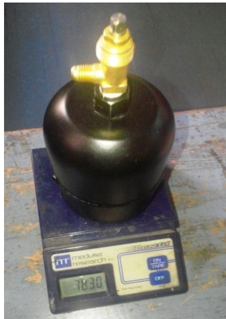
Fig 5.6: Measurement of Percentage of Lubricating Oil Mixing
