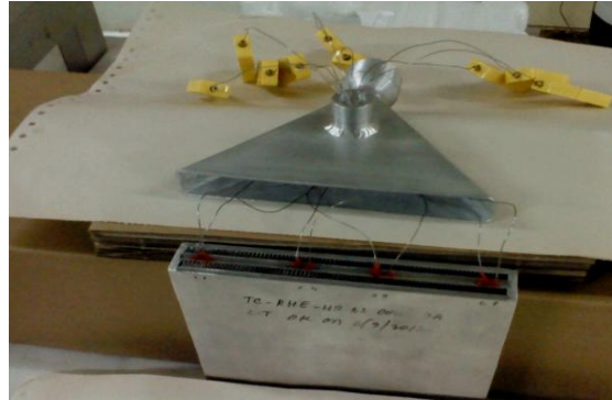
Fig. 4.8: Photograph Showing Thermocouples Fixing Arrangement in Test Condenser Core
