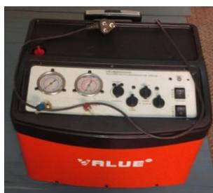
Fig. 4.26: Photograph of Test Rig Evacuation and Refrigerant Charging Unit
