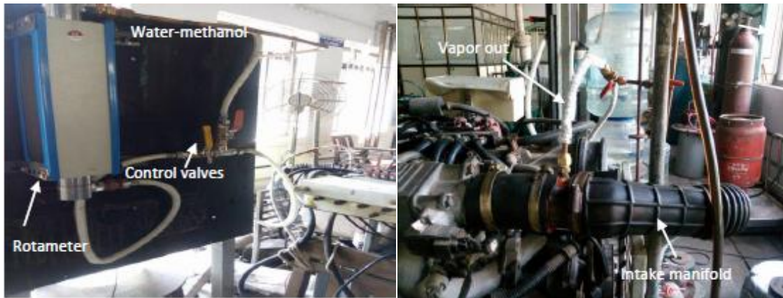
Fig. 4.10 Photographs of Vaporized Water-Methanol Injection System
