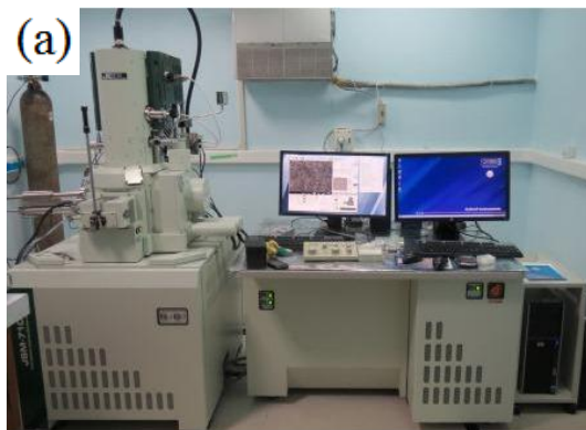
Figure 3.11 (a) FE-SEM (b) Struers electro polishing machine
