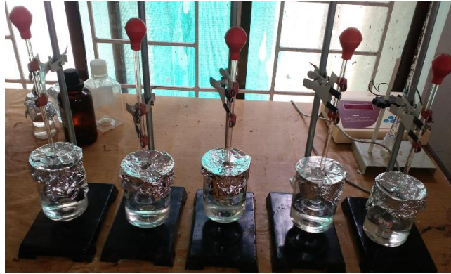
Figure 3.20 Immersion test setup
