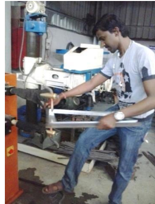
(b) Welding of the plates
