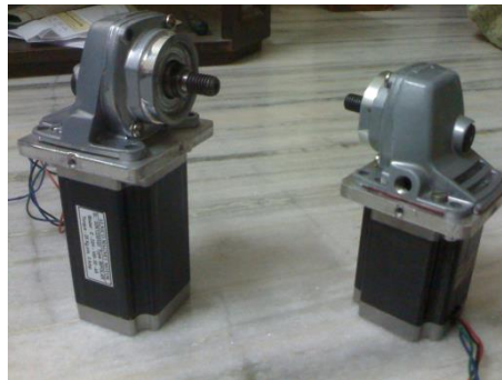
Fig.3.34 Hybrid NEMA Make High Torque Motors M_1 and M_2
