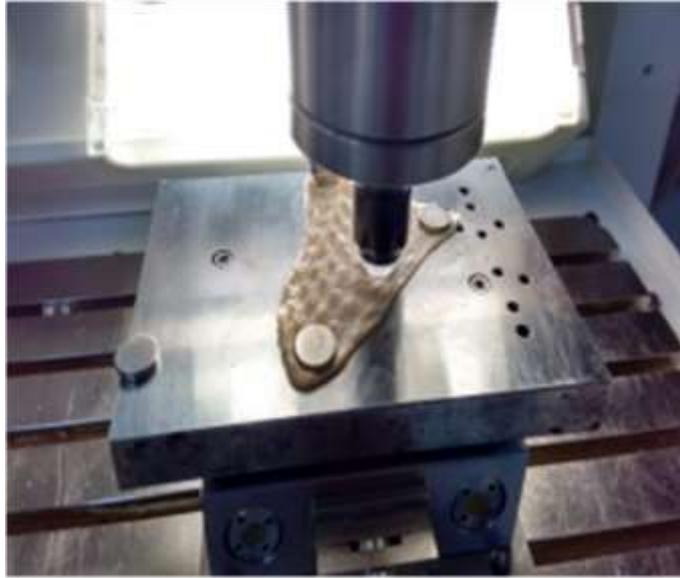
**Figure 4.40** Test Setup for Piercing Chicken Skin by Microneedle
