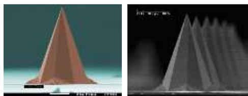
**Figure 2.16** 400  $\mu\text{m}$  Tall Silicon Microneedles (www.tyndall.ie)
