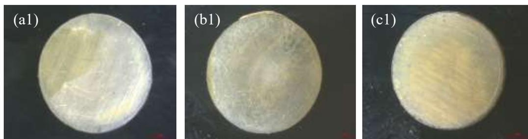
**Figure 5.15** Images of Roughened Surface With Different Grit papers (220, 500, and 1000) after coating
