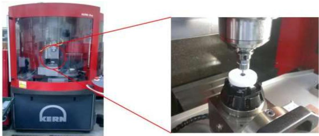
**Figure 4.16** Micro-Holes Drilling on Micromachining Centre
