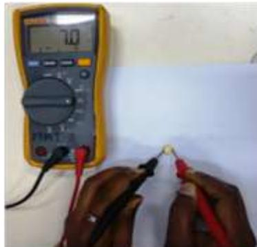
**Figure 5.20** Resistance Measurement
