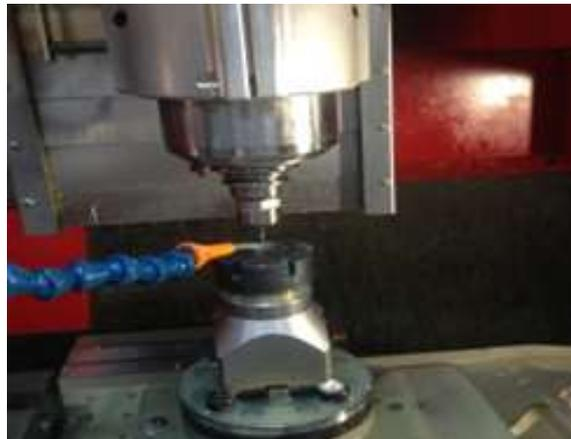
**Figure 4.24** Microneedle Machining Setup With High-Speed Milling Spindle
