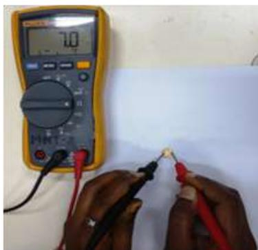
**Figure 4.41** Electrical Resistance Measurement Using Multimeter
