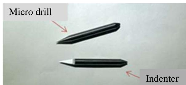
**Figure 4.14** Carbide Micro-Indenter and Micro-Drill
