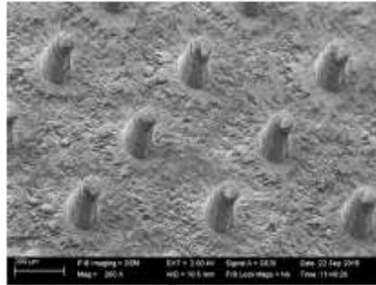
**Figure 4.35** SEM Image of Compressed Microneedles
