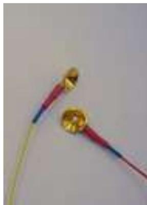
**Figure 1.5** Cup Electrodes for Measurement of EEG
