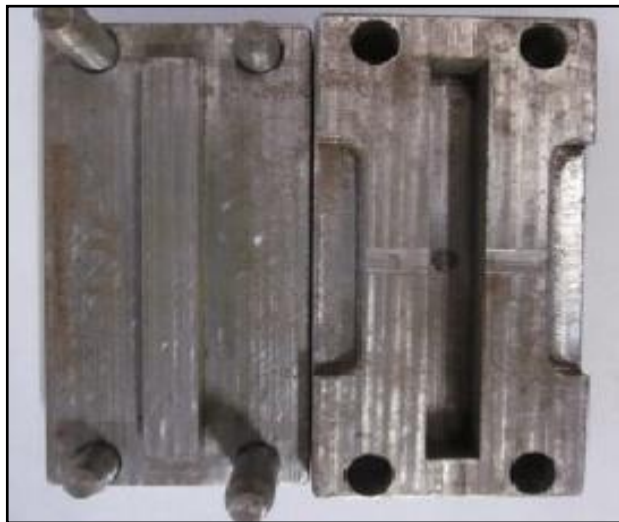
Figure 2.9: Open flash type compression mould for flexural and wear samples
