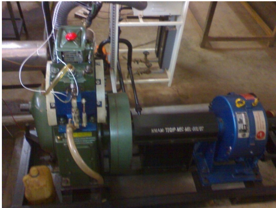
Figure 3.11 Photograph of VCR Diesel engine test rig
