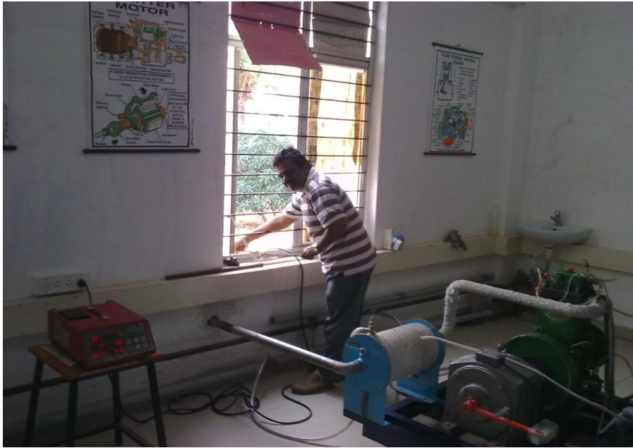
Figure 3.9 Photograph of the exhaust gas analyzer probe at engine exhaust
