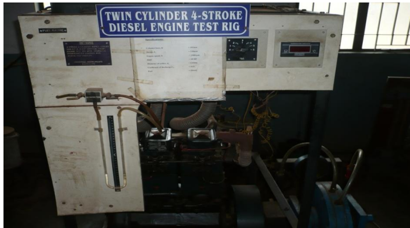
Figure 3.13 Photograph of Twin cylinder diesel engine test rig
