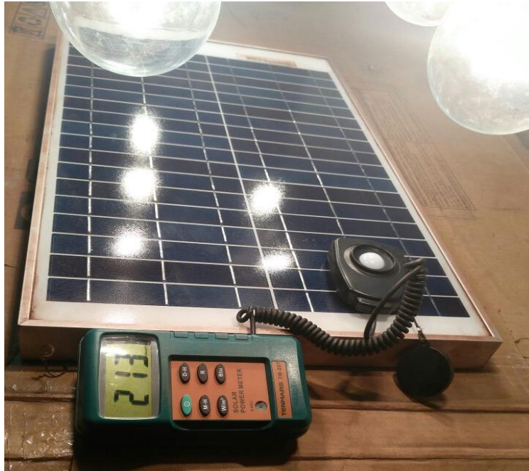
Figure 4.3 Measurement of solar radiation falling on the PV panel surface
