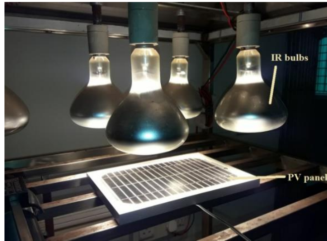
Figure 7.1 Heating of PV panel surface
