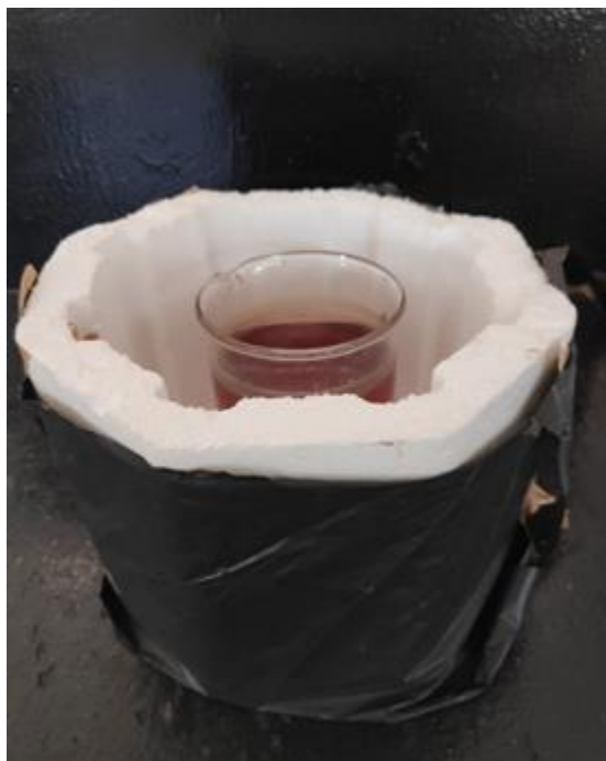
Fig. 3.1 Beaker containing \text{Co}_3\text{O}_4 nanofluid in thermo cool
