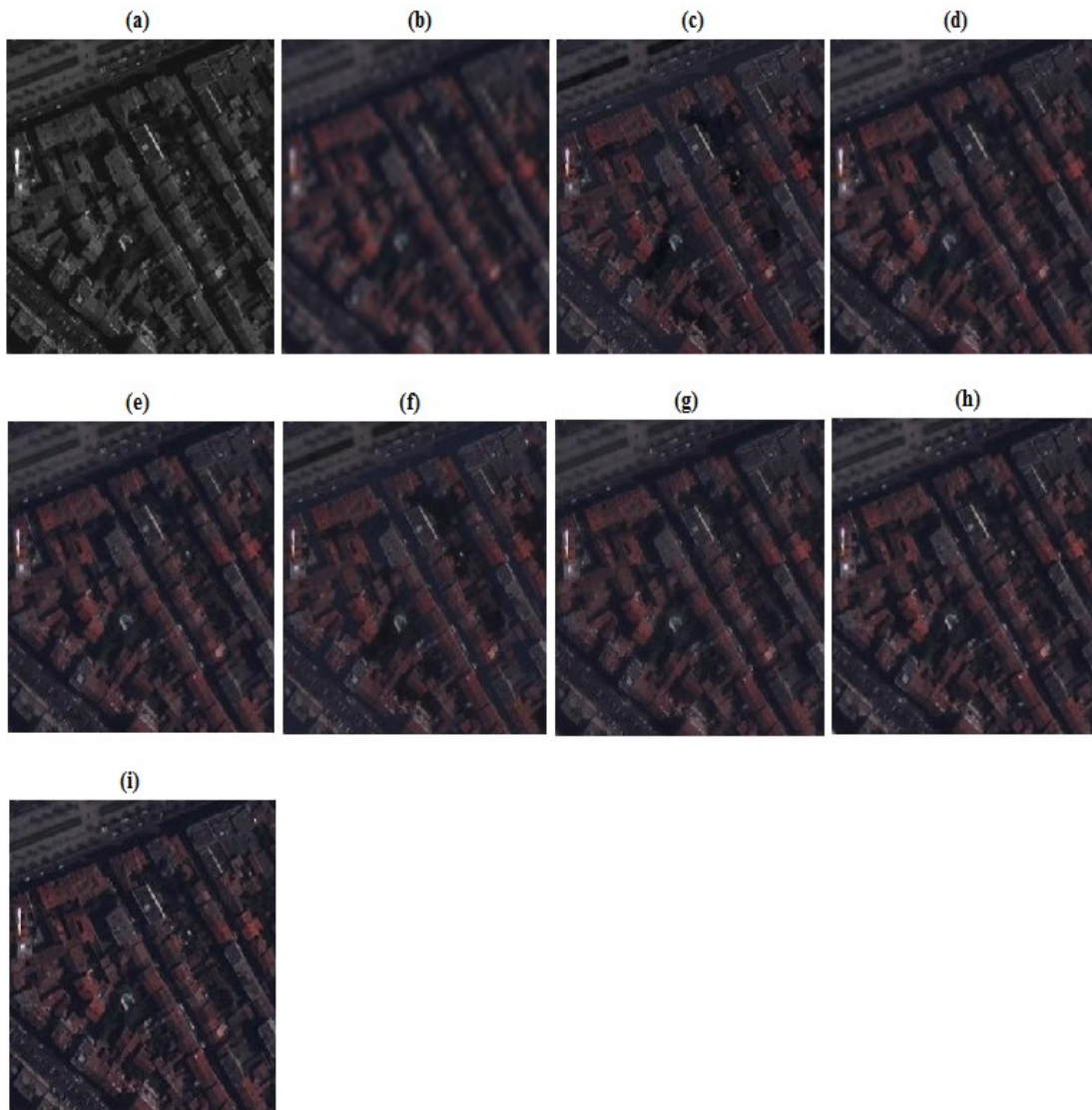
Figure 3.7: Pan-sharpening results evaluated using QNR protocol for Pléiades data (a) PAN image ( 256 \times 256 , simulated) (b) Up-sampled MS image ( 256 \times 256 , 60-cm) (c) FIHS (d) AWLP (e) SR-Li (f) SR-TD (g) SR-WT (h) SR-D (i) Proposed method
