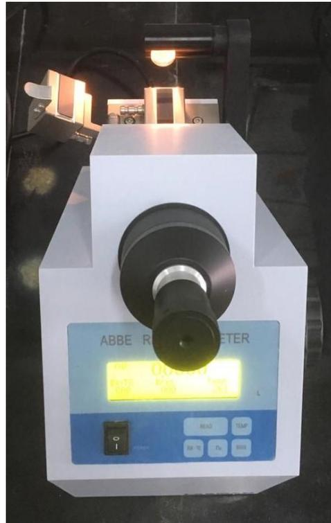
**Figure 2.4: Abbe Refractometer**
