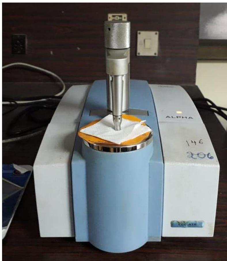
**Figure 2.3: FTIR Spectrometer**
