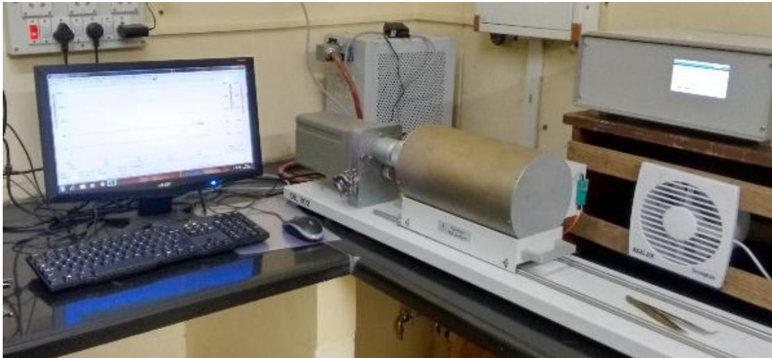
**Figure 2.5: TA DIL802 differential dilatometer**
