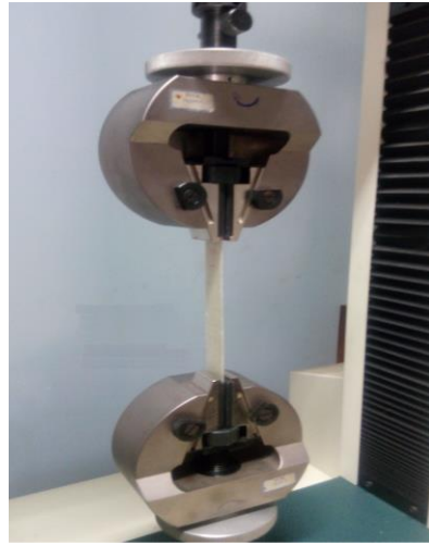
Figure 5.2 Experimental tensile setup
