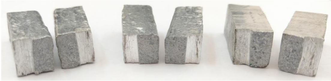
Figure 7.11 Impact test specimens of Al6082 as-cast alloy
