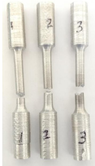
Figure 7.9 Tensile test specimens of as-cast Al6082 alloy
