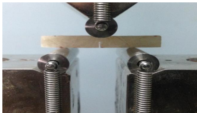
Figure 5.10 Fracture toughness testing in UTM
