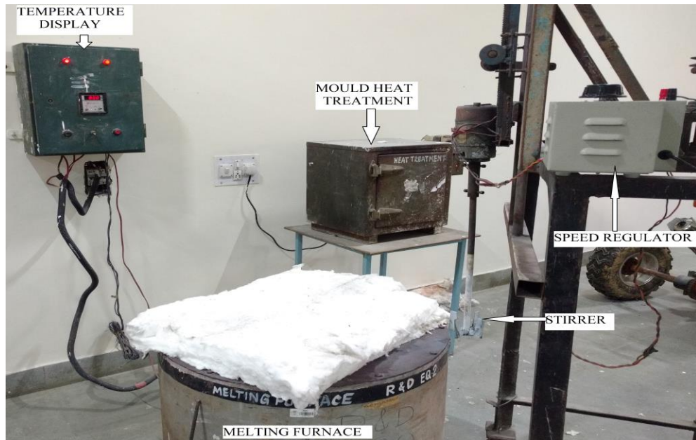
Figure 3.13 MMCs stir casting experimental setup
