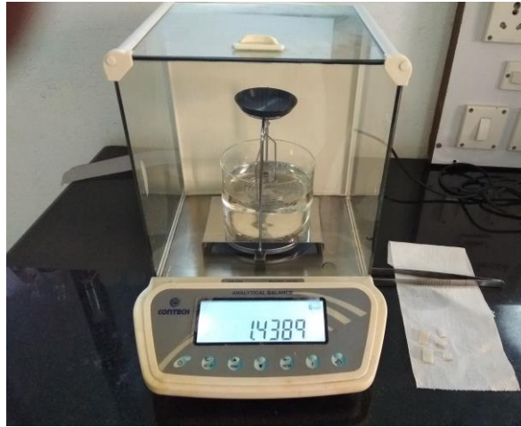
Figure 5.1 Density measurement kit
