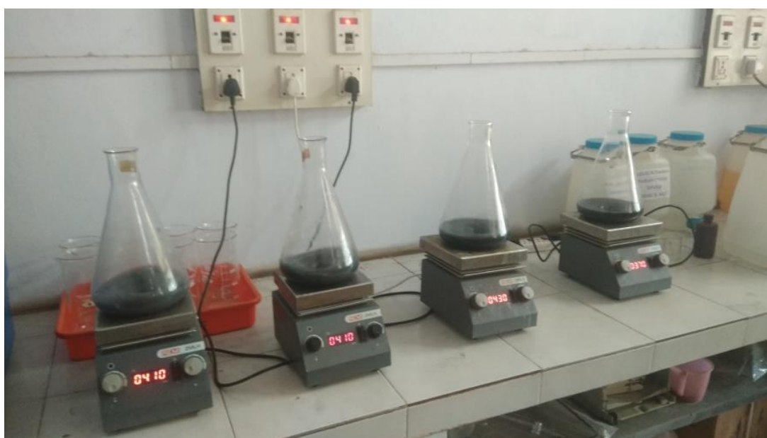
Figure 4.6 Experimental set up for finding optimum condition for the removal of COD
