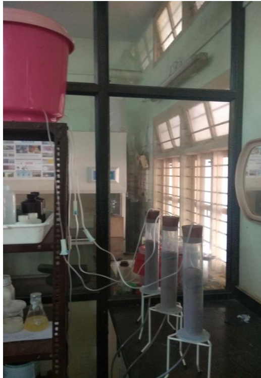
Figure 4.9 Experimental Setup for the fixed-bed adsorption study
