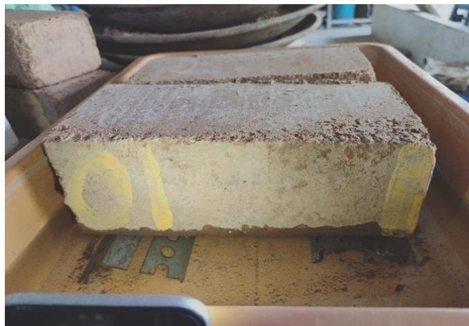
Fig. 7.10 Initial rate of water absorption test
