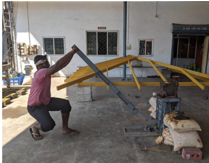
Fig. 7.1 Compressing the block by pulling down the lever arm
