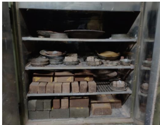
Fig. 7.4 Oven drying of CSEBs
