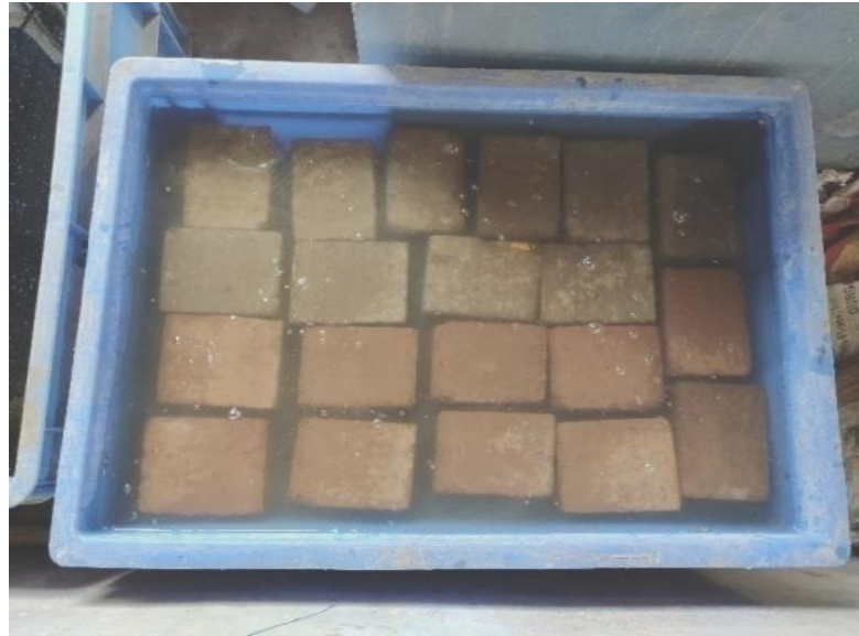
Fig. 7.8 Water absorption test on CSEBs
