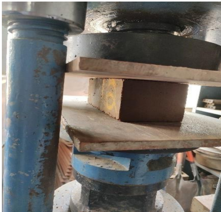
Fig. 7.5 Compression test of CSEB
