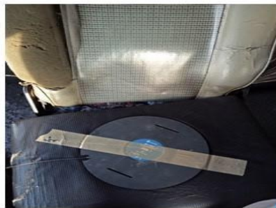
Fig. 3.2 The Svantek SV 38V seat pad fixed to the seat-surface using duct tape
