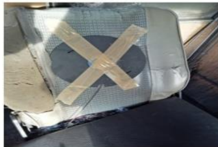
Fig. 3.3 The Svantek SV 38V seat pad fixed to the seat-back using duct tape
