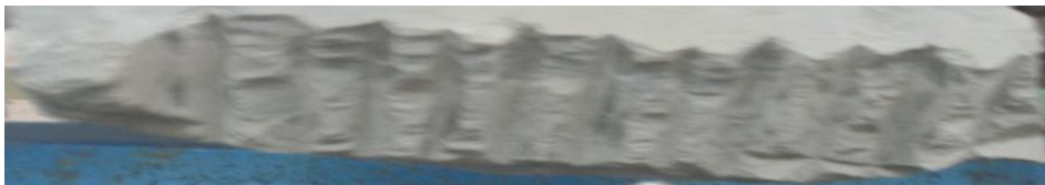
Figure 3.17 The groove which is formed during the cutting of sandstone.
