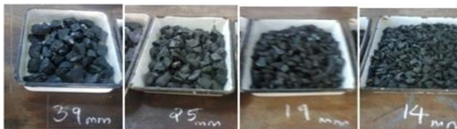
Figure 3.4 Specimen prepared for Los Angeles abrasion test
