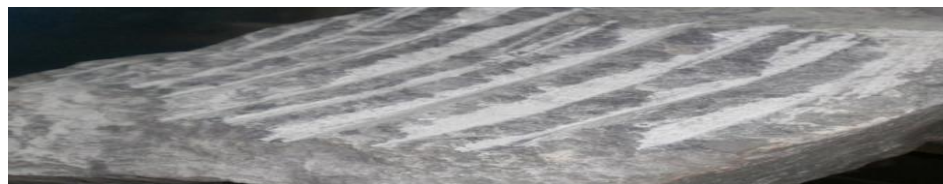
Figure 3.18 The groove which is formed during the cutting of limestone.
