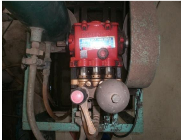
Figure 3.14 Hydraulic unit for the rock cutting machine
