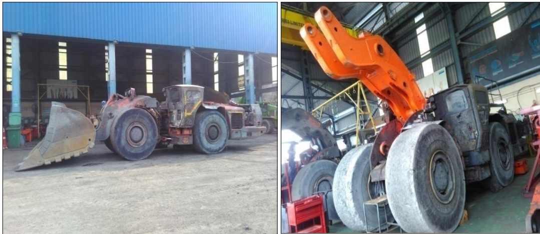
Figure 3.1 (a) and (b) LH517 model LHD machine at a workshop for maintenance
