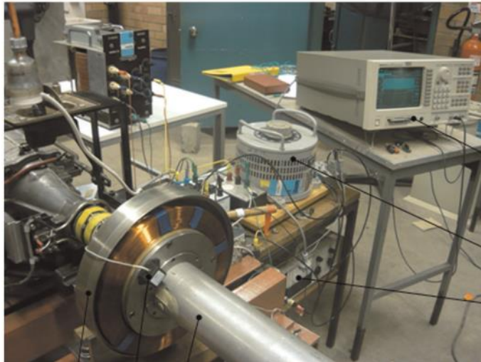
Figure 2-8: MR Elastomer based torsional Vibrations absorber
