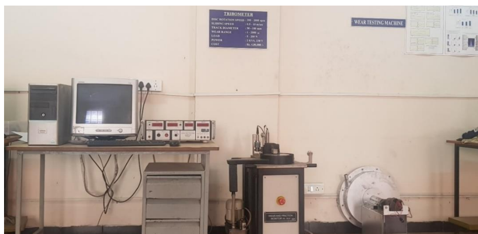
Figure 3.8 DUCOM Wear Testing Machine
