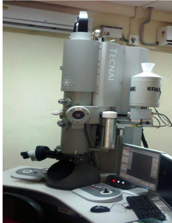
Figure 3.2 TECHNAI Transmission Electron Microscopy set-up
