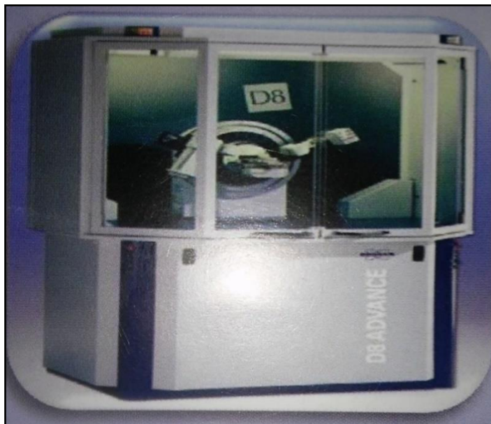
Figure 3.4 D8 Advance X-Ray Diffraction set-up
