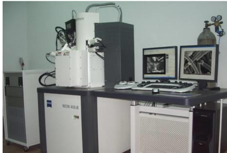
Figure 3.3 Carl Zeiss Scanning Electron Microscopy set-up
