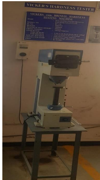
Figure 3.7 Vickers Hardness Tester
