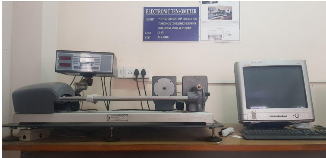
Figure 3.6 PC-2000 Electronic Tensometer
