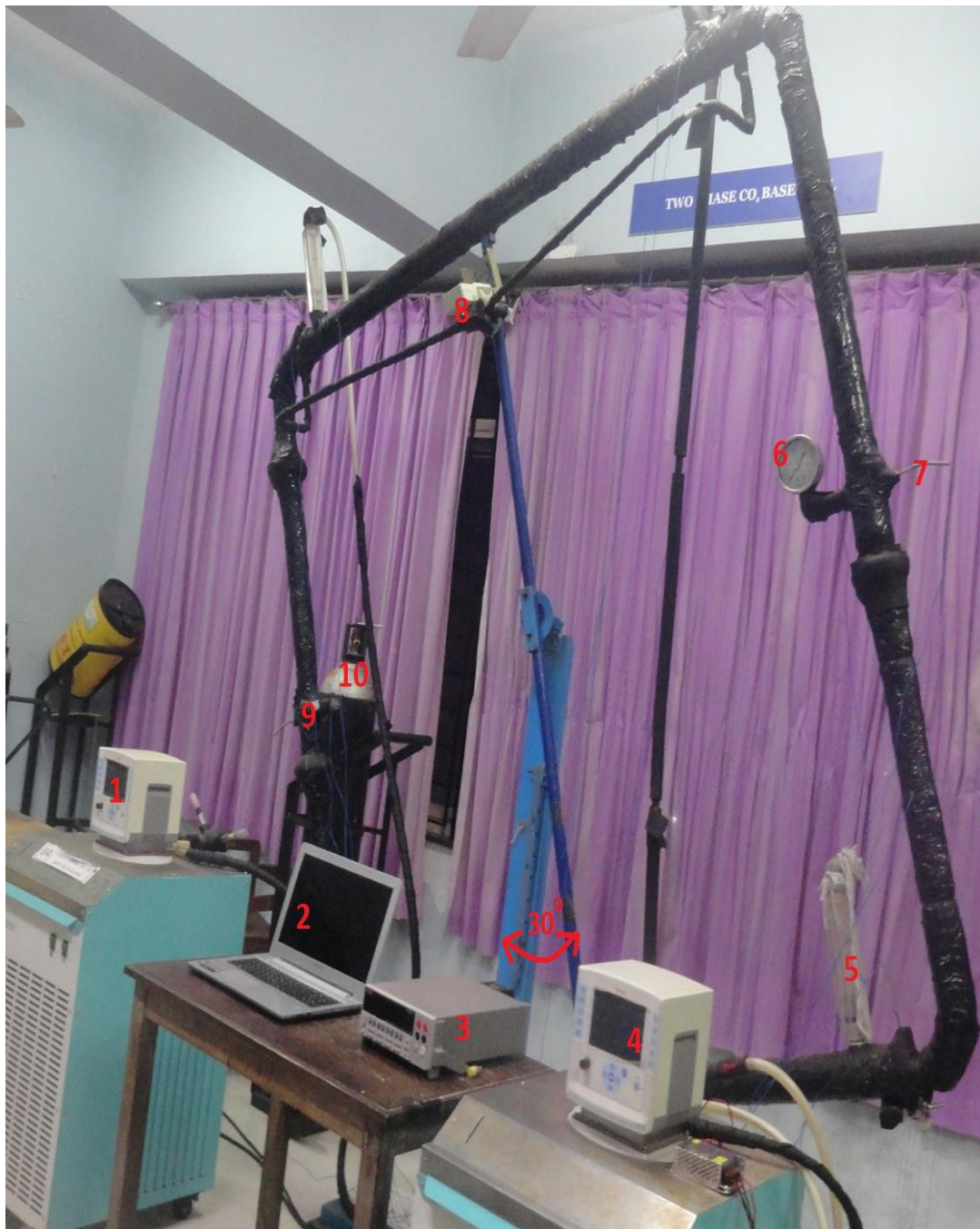
1:Thermostatic bath- 1(HHX), 2: Computer to read DAQ data, 3: DAQ (Data acquisition system), 4: Thermostatic bath -2(CHX), 5: Rotameter, 6: Pressure Gauge, 7: T-Type thermocouple, 8: Differential Pressure Transducer, 9: Safety Valve, 10: CO 2 cylinder.
