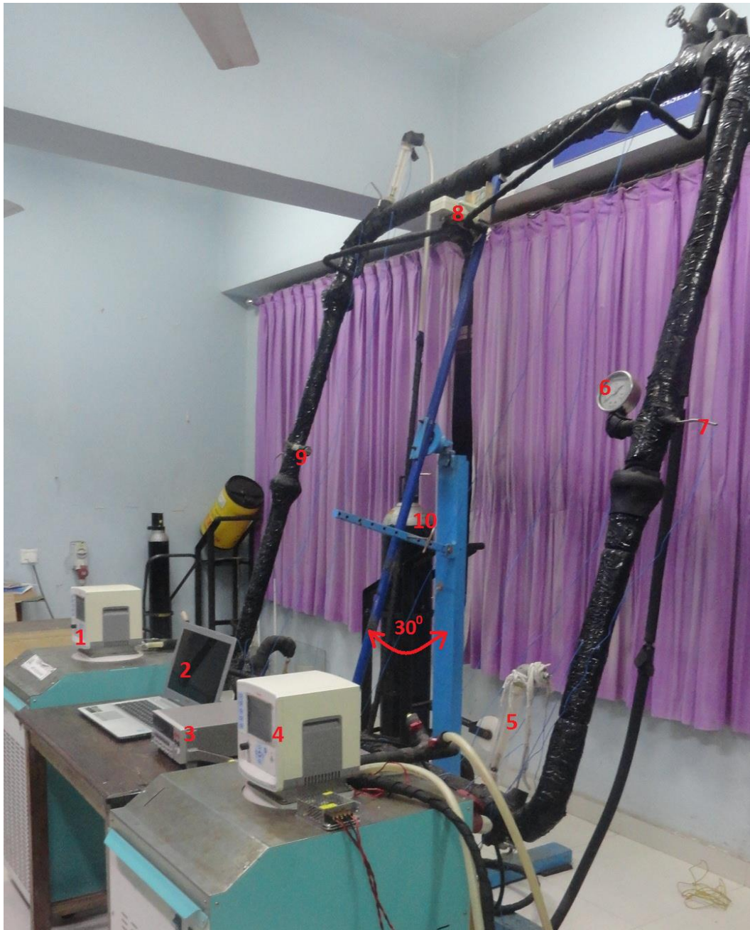
1:Thermostatic bath- 1(HHX), 2: Computer to read DAQ data, 3: DAQ (Data acquisition system), 4: Thermostatic bath -2(CHX), 5: Rotameter, 6: Pressure Gauge, 7: T-Type thermocouple, 8: Differential Pressure Transducer, 9: Safety Valve, 10: CO 2 cylinder.
