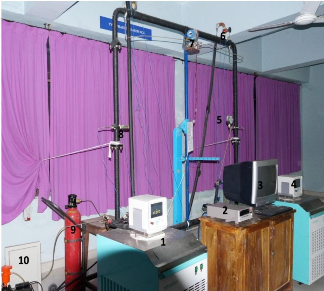
1: Thermostatic bath- 1(HHX), 2: DAQ, 3: Computer to read DAQ Data, 4: Thermostatic bath -2(CHX), 5: Pressure Gauge, 6: Rotameter, 7: Differential Pressure Transducer, 8: Safety Valve, 9: CO 2 cylinder, 10:Vaccum pump.
