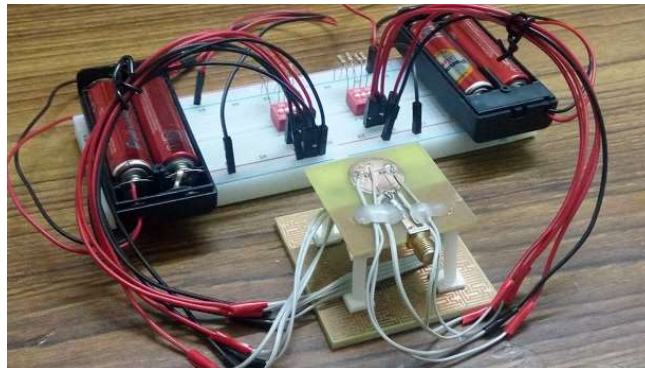
Fig. 6.19: Biasing circuit for antenna backed by metasurface
