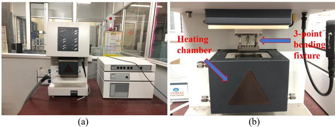
Figure 2.15. (a) Dynamic mechanical analyser apparatus and (b) 3-point bending configuration.
