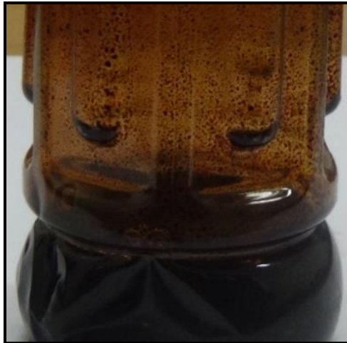
Fig. 5.8 Gummy deposits formed during storage of CTPO
