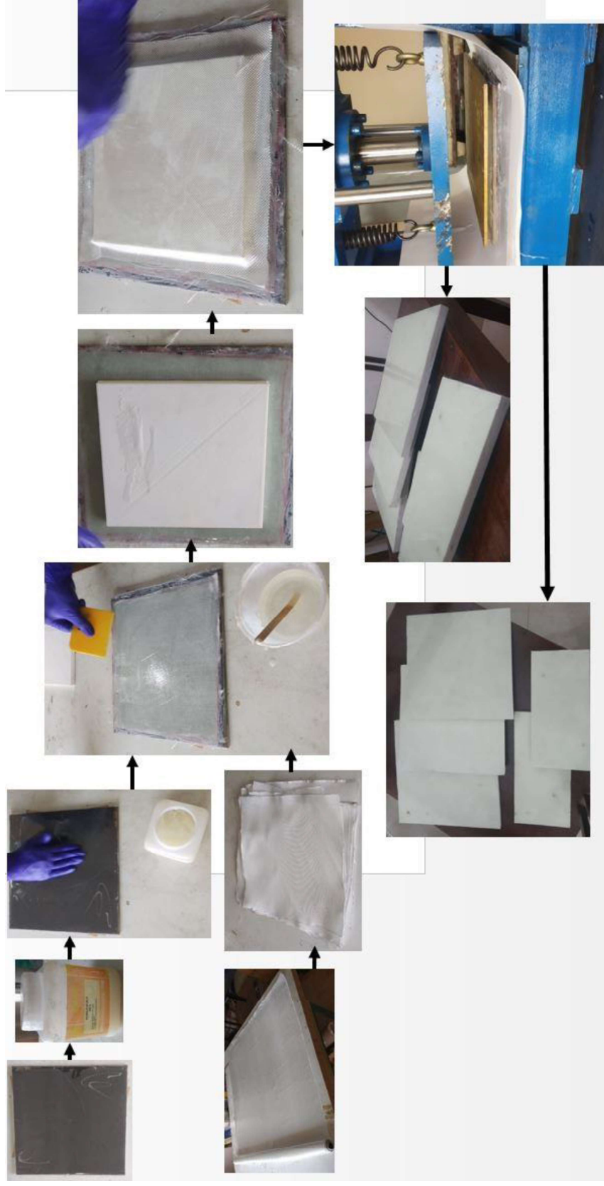
Figure 7.2: Graphical representation of fabrication of LCS plates with 3D printed PLA core.
