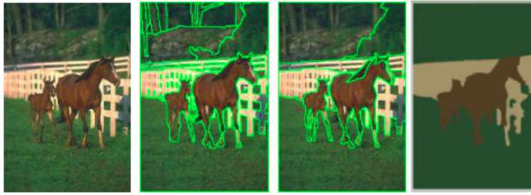
Figure 3.23: Sample images of different stages of proposed MRF-CRP model for weakly supervised image segmentation
