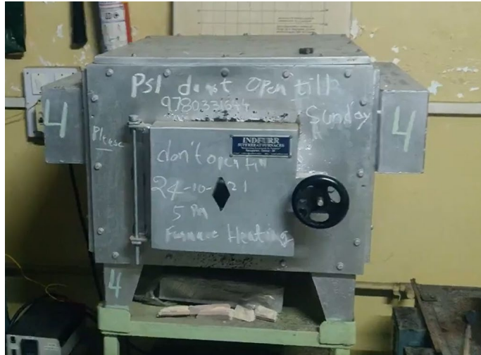
Figure 3.3 Furnace used to carry out high temperature oxidation experiments
