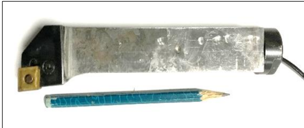
Figure 7.7 Assembled image of the fabricated tool holder
