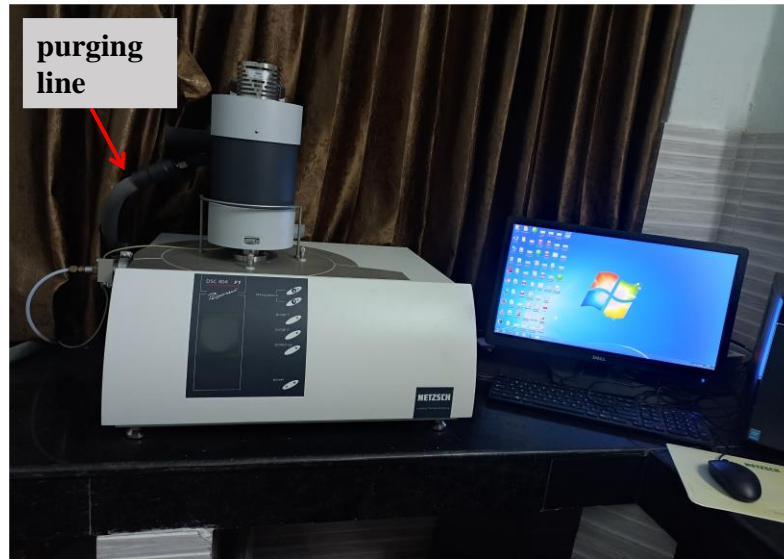
Figure 2.6 DSC test setup.
