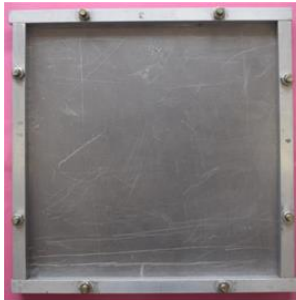
Figure 2.8 Casting mold for the sample fabrication.
