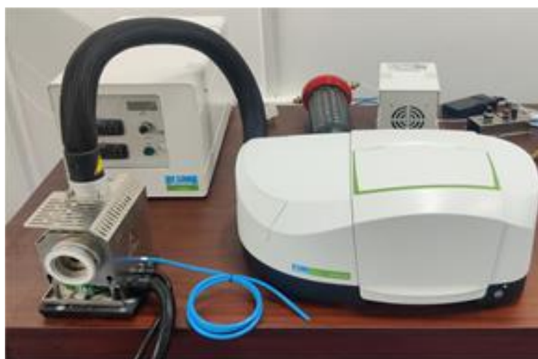
Figure 2.4 FTIR spectroscopy test setup.
