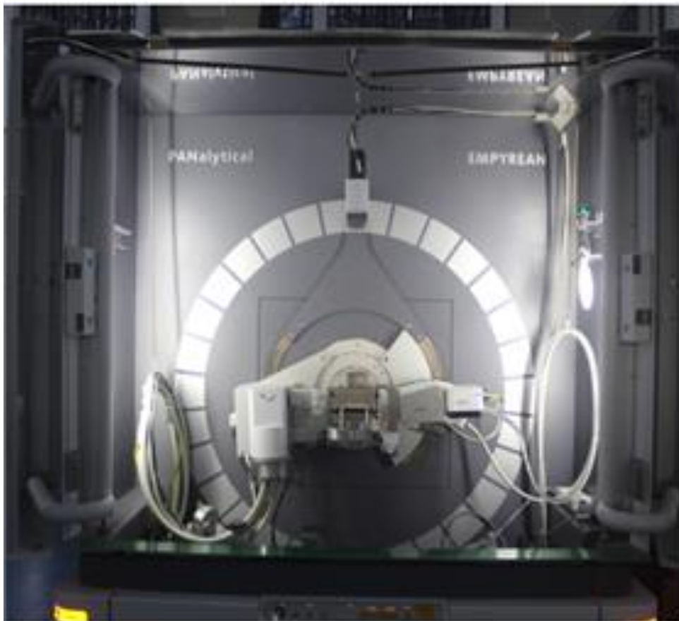
Figure 2.5 XRD test setup.
