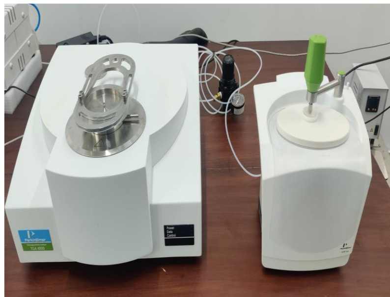
Figure 2.7 TG analysis setup.
