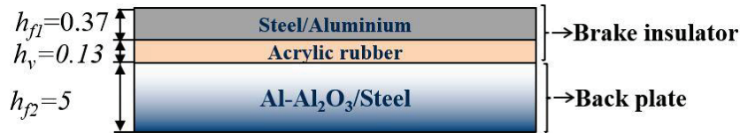
Figure 5.2: Back plate with brake insulator.
