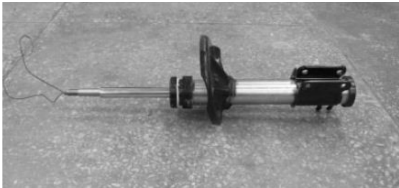
Figure 2.4 MR damper developed for quarter car testing and analysis ( Courtesy: Sung & Choi (2008) )
