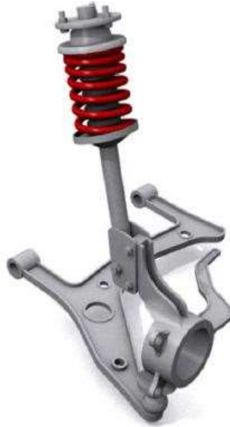
Figure 3.1 Suspension scheme in McPherson strut ( Courtesy: Fallah et al. (2009) )
