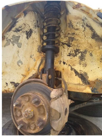
Figure 6.2 MR damper in the McPherson strut system in the vehicle
