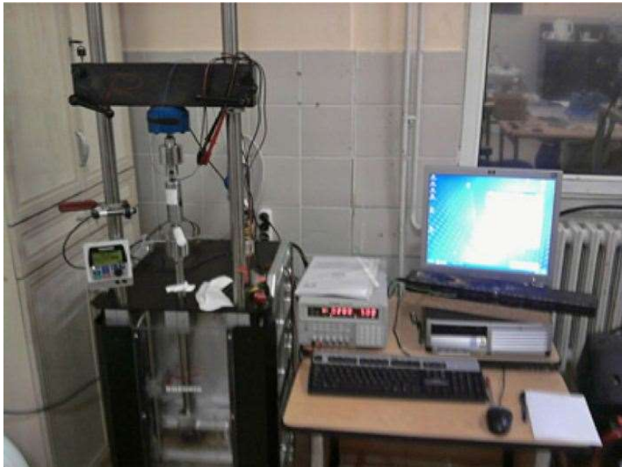
Figure 2.5 Damper testing setup (Courtesy: Parlak and Engin (2012))
