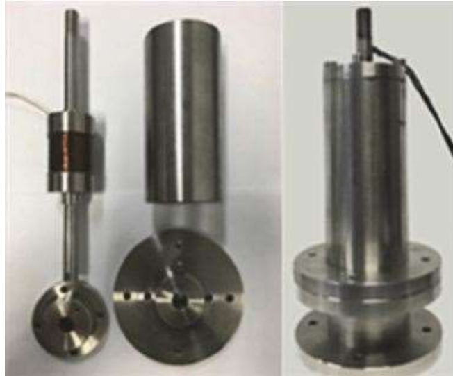
Figure 2.6 A shear mode monotube MR damper ( Courtesy: Meng & Zhou (2019) )
