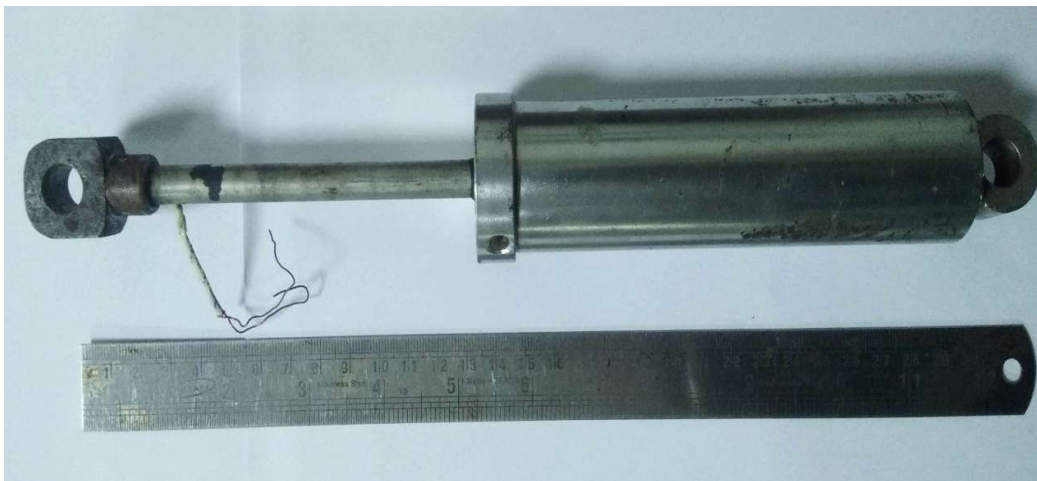
Figure 3.9 Fabricated MR damper (prototype-1)
