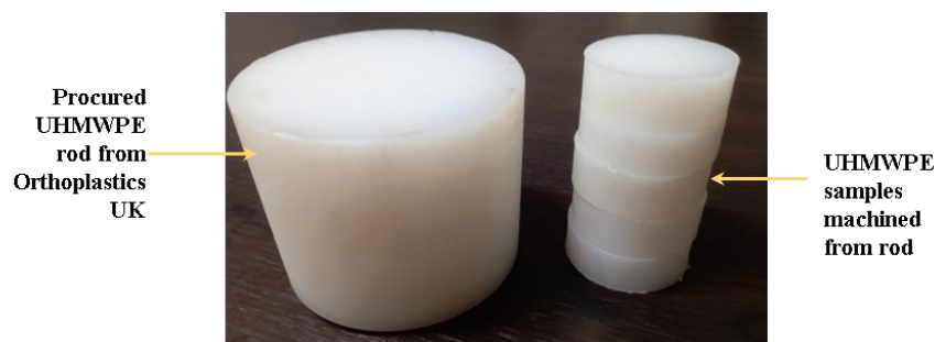
Figure 8.2 Samples prepared from ram extruded UHMWPE by CNC machining
