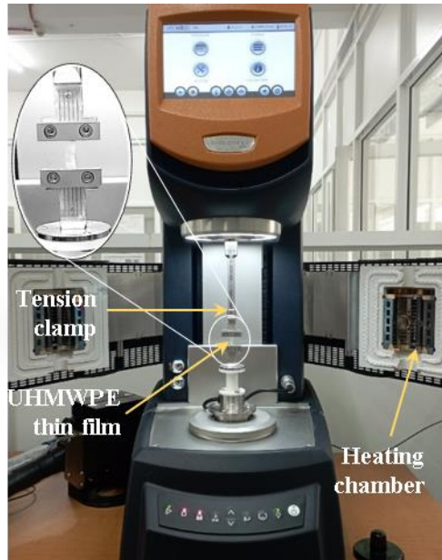
Figure 8.14 The DMA analysis of UHMWPE thin film using a dynamic hybrid rheometer
