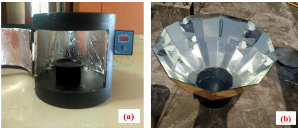
Figure 3.7 (a) Cylindrical box solar cooker with cooking vessel (b) cooker fitted with decahedron reflector
