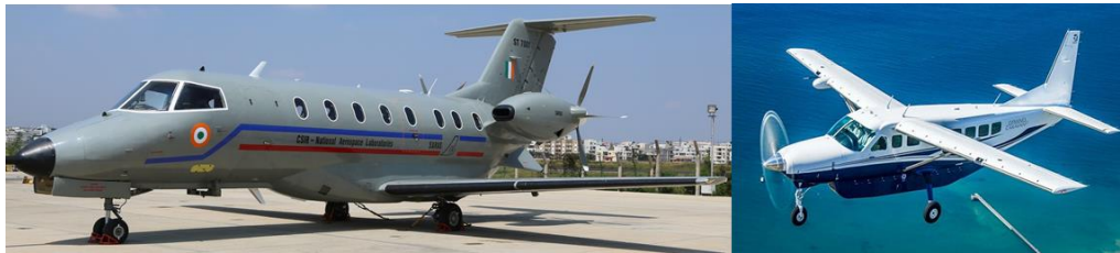
Figure 1.10 Aircraft with a) Pusher configuration b) Tractor configuration
