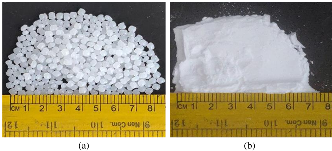
Figure 2.1. Representative picture of as received (a) HDPE and (b) Hollow GMB.
