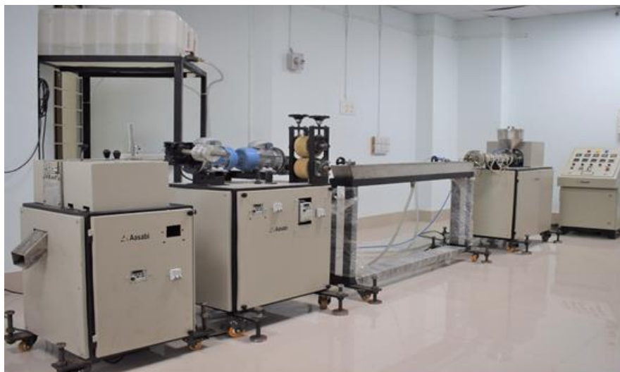
Figure 2.6. Experimental setup of extruder.
