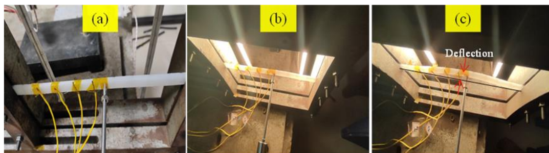
Figure 7.10. 3DP HDPE sample (a) Before testing (b) while testing and (c) post buckling.
