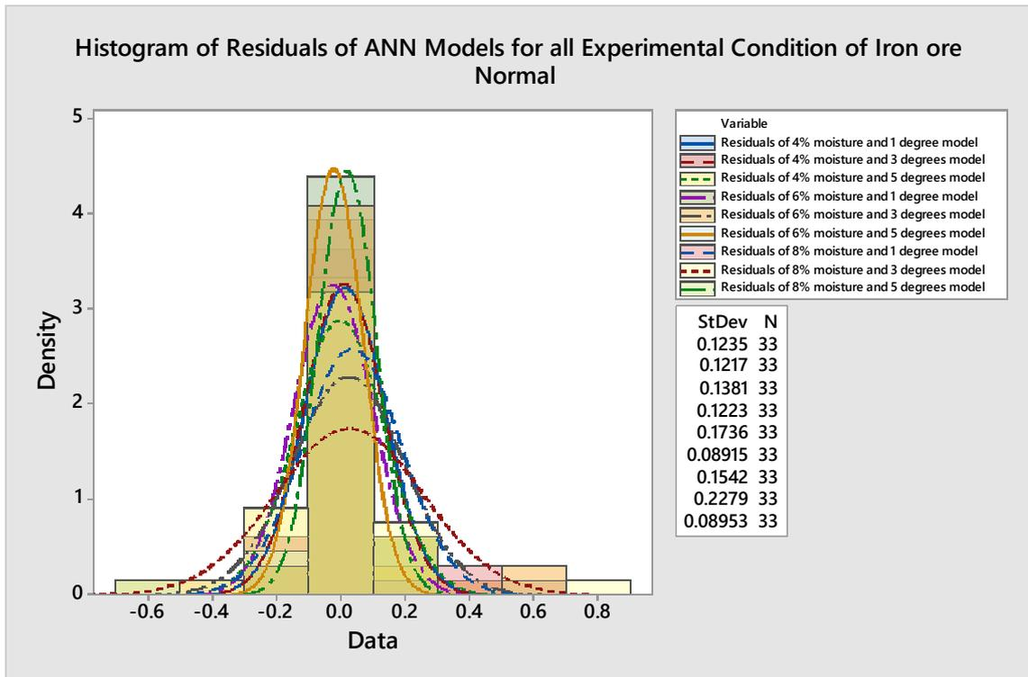
Fig. 4.23 Histogram of residual of ANN models for all the experimental conditions of iron ore
