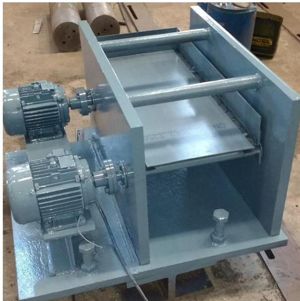
Fig. 4.30 Final assembly of the flexible screening machine as a feeder
