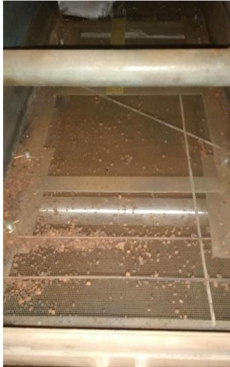
Fig. 4.11 Clogging of iron ore
