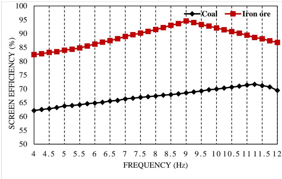
Fig. 4.3 Vibratory screen efficiency of coal and iron ore maintained at 4% moisture and 5°
