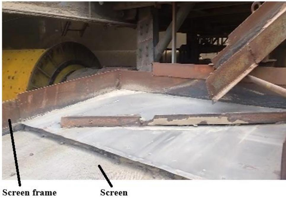
Fig. 3.3 Screen connected to the screen frame with fasteners
