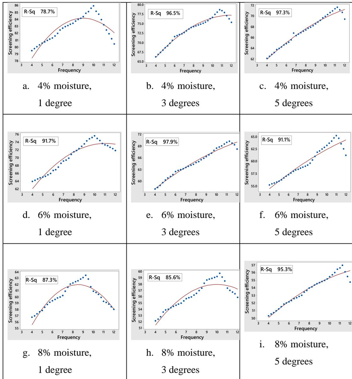
Fig. 4.12 Regression data fitting results for all the conditions of screening coal
