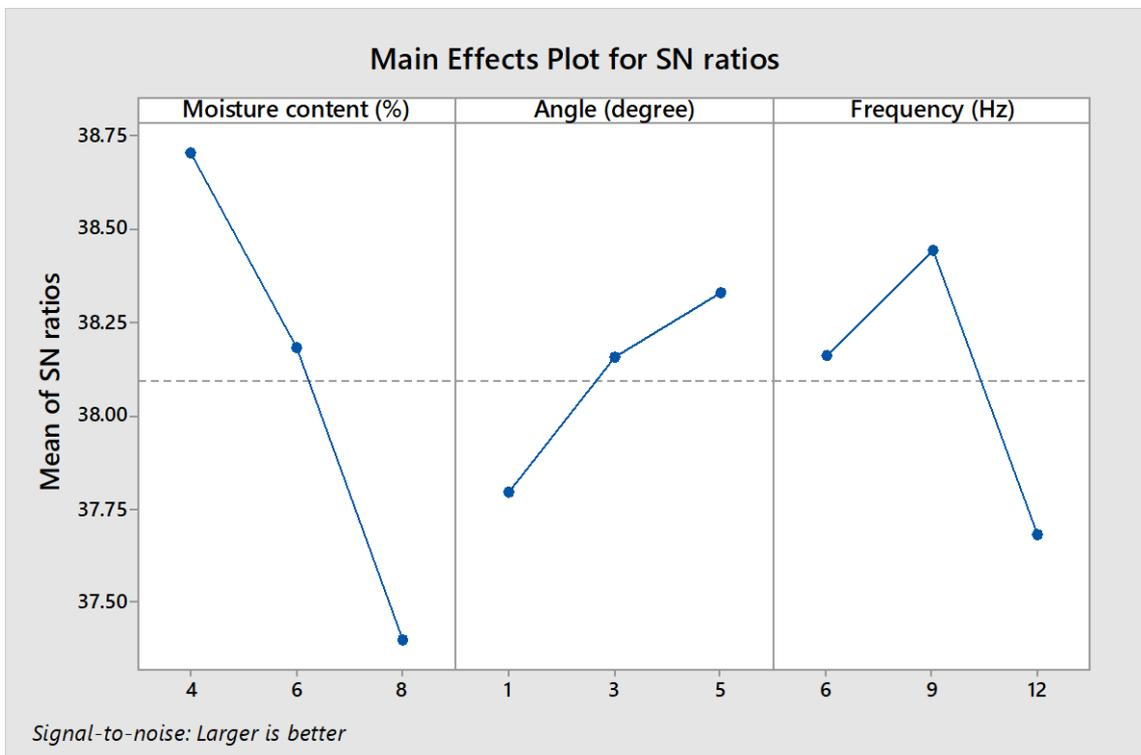
Fig. 4.25 Main effect plot obtained for moisture content, angle, and frequency on iron ore screening performance
