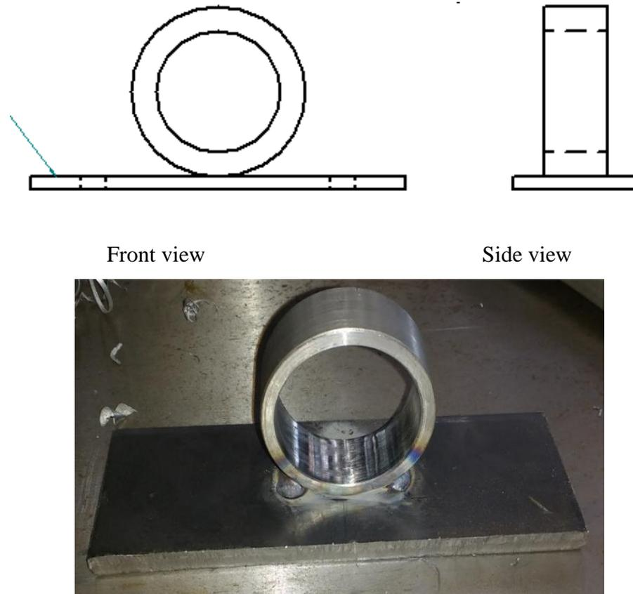
Fig. 3.8 Front view, side view and fabricated part of the screen holder
