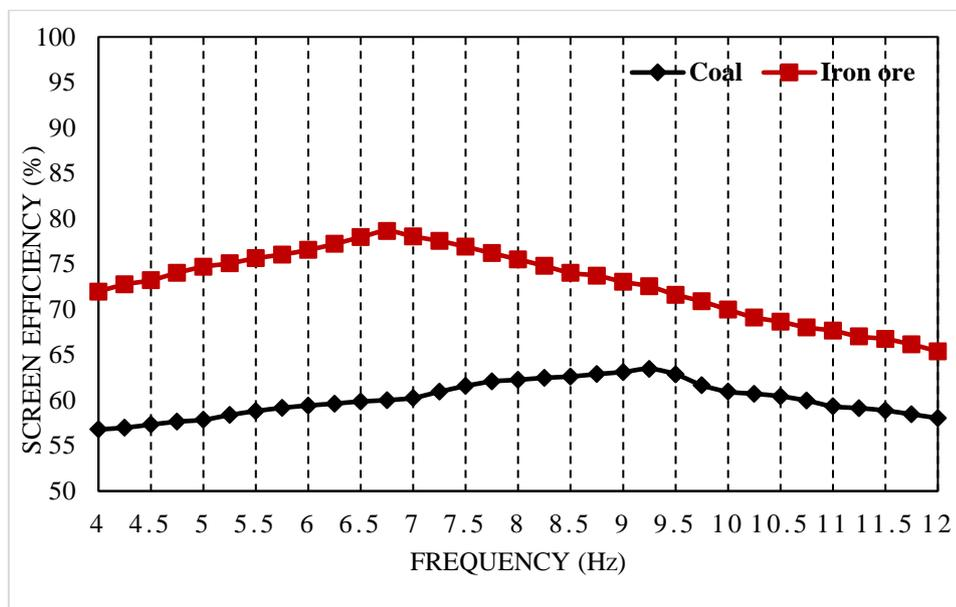
Fig. 4.7 Vibratory screen efficiency of coal and iron ore maintained at 8% moisture and 1°
