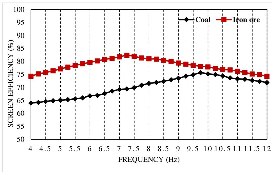
Fig. 4.4 Vibratory screen efficiency of coal and iron ore maintained at 6% moisture and 1°
