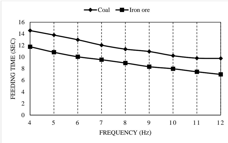
Fig. 4.31 Feeding performance of coal and iron ore
