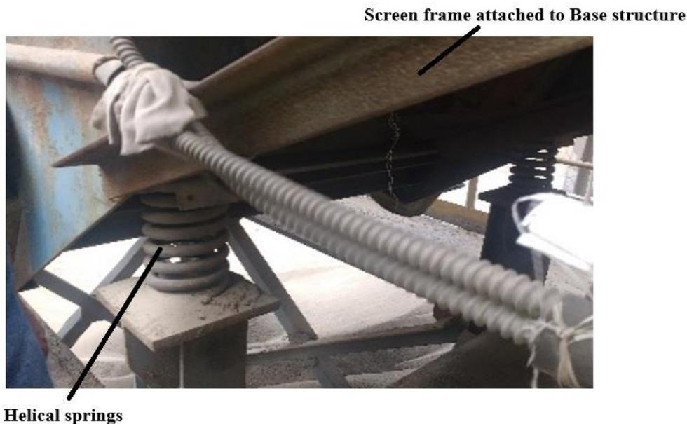
Fig. 3.5 Helical springs attached between the screen frame and base structure
