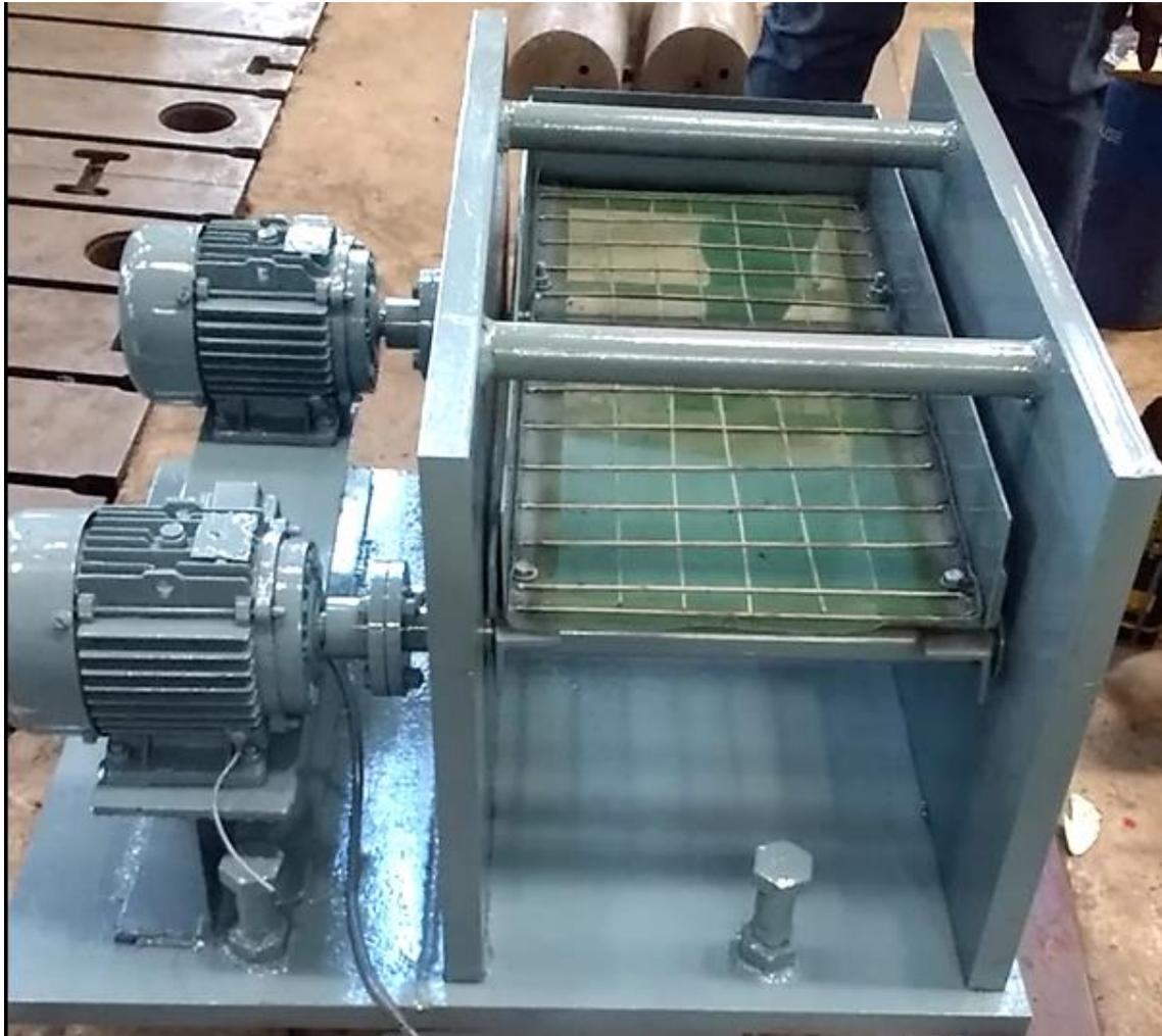
Fig. 3.17 Final assembly of the flexible screening machine
