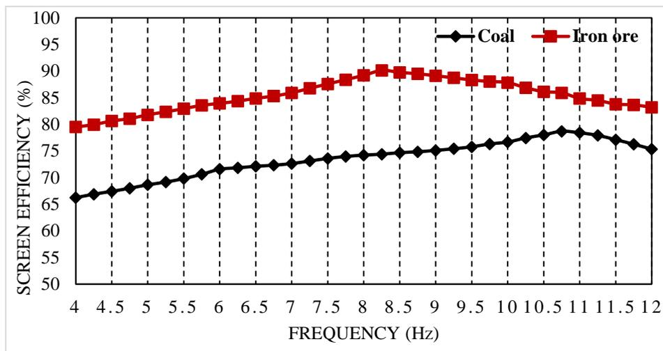
Fig. 4.2 Vibratory screen efficiency of coal and iron ore maintained at 4% moisture and 3°
