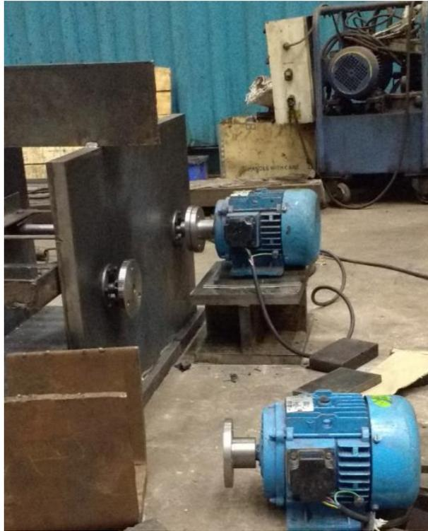
Fig. 3.15 Assembly of the eccentric shafts to the respective motors
