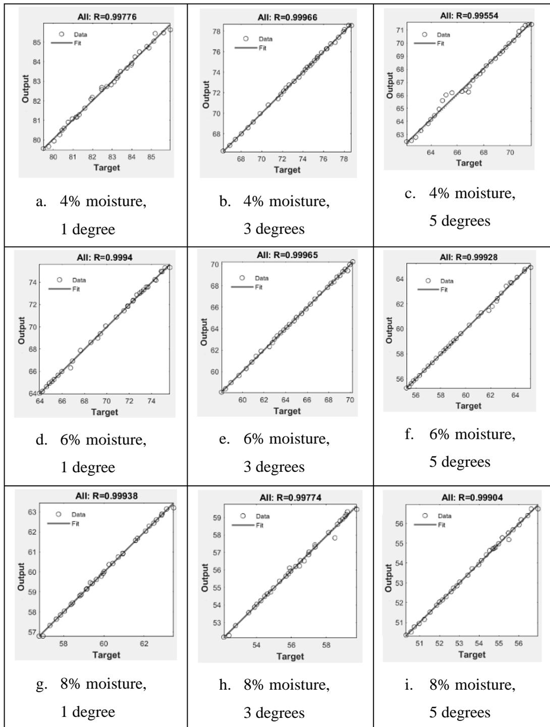
Fig. 4.14 ANN overall data fitting results for all the conditions of screening coal
