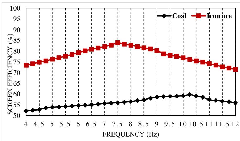
Fig. 4.8 Vibratory screen efficiency of coal and iron ore maintained at 8% moisture and 3°
