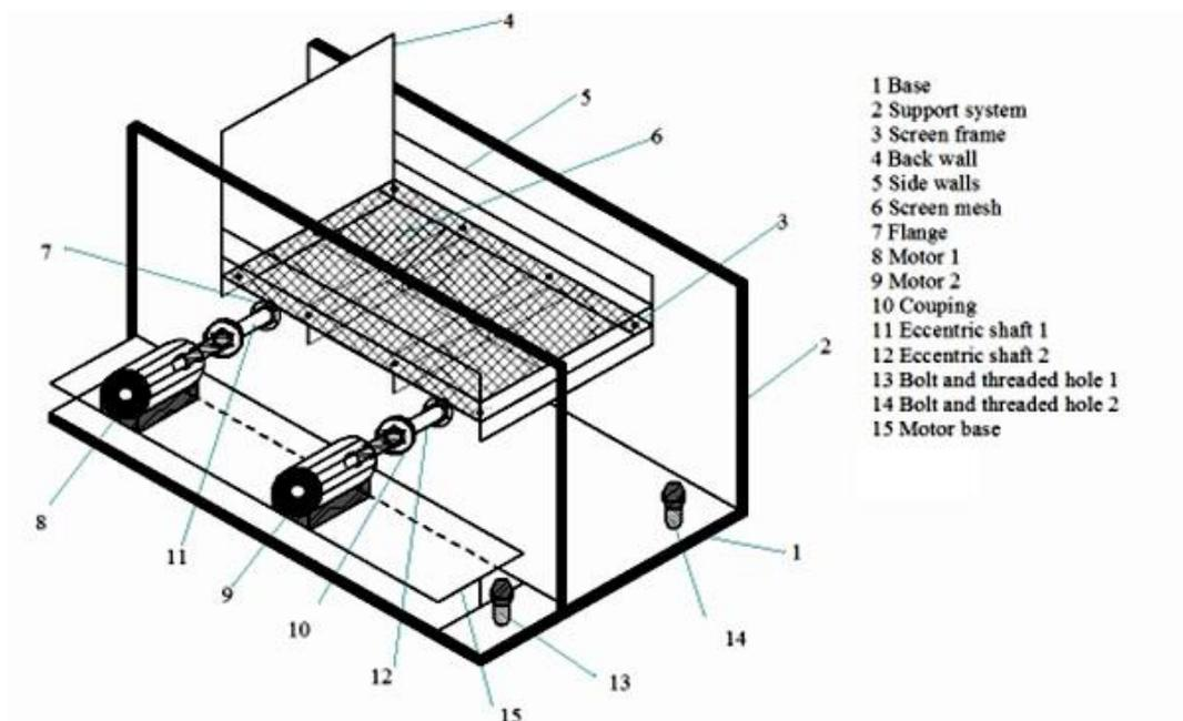
Fig. 3.16 Final assembly drawing of the flexible screening machine
