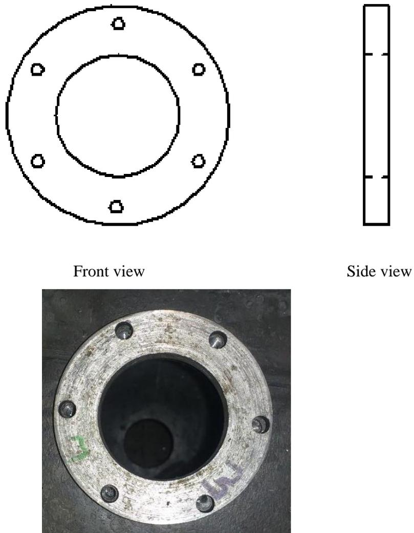
Fig. 3.6 Front view, side view and fabricated part of the flange
