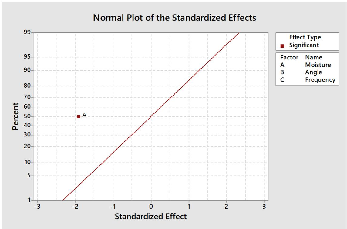
Fig. 4.28 Normal plot for screening coal using fractional factorial design
