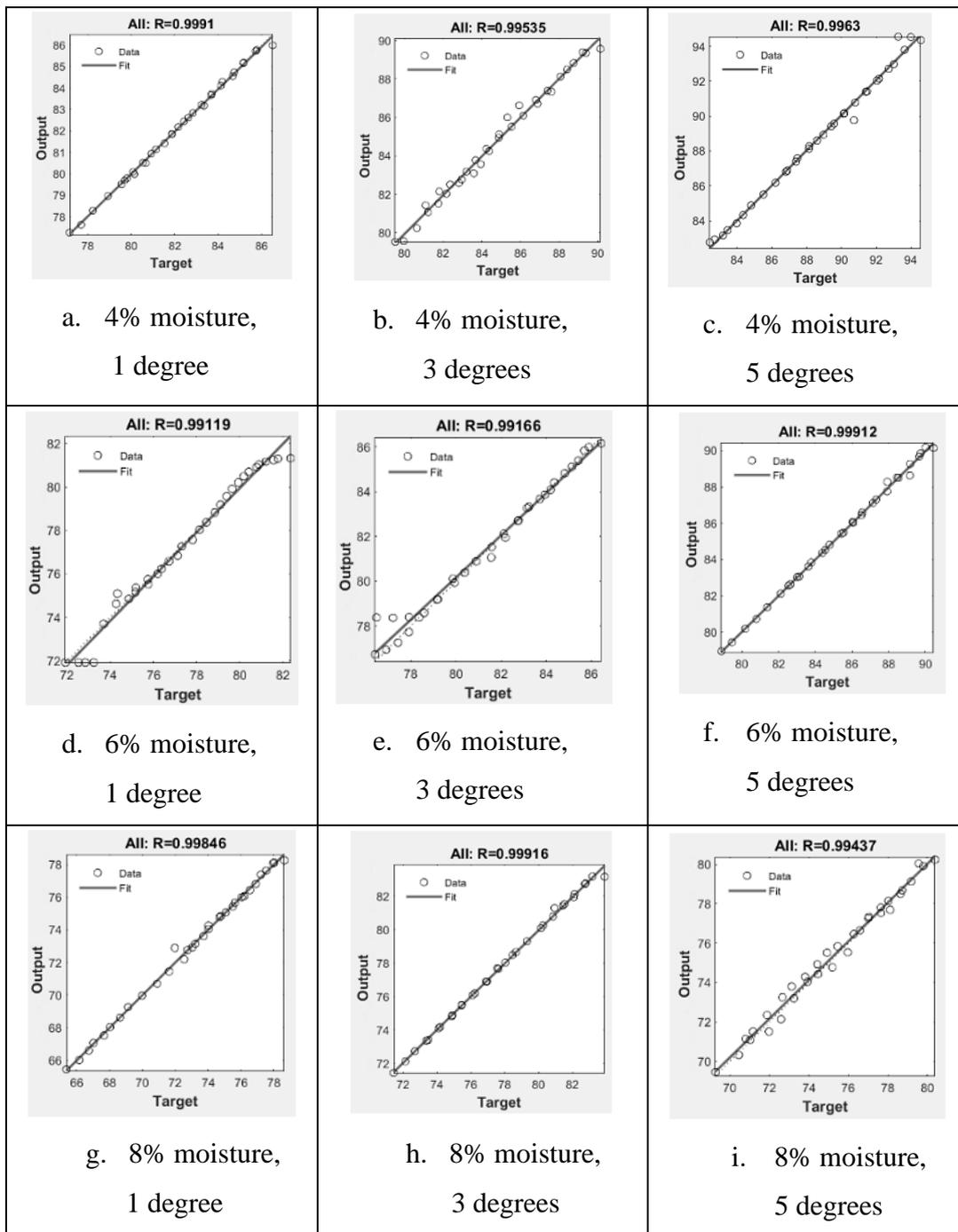
Fig. 4.15 ANN overall data fitting results for all the conditions of screening iron ore
