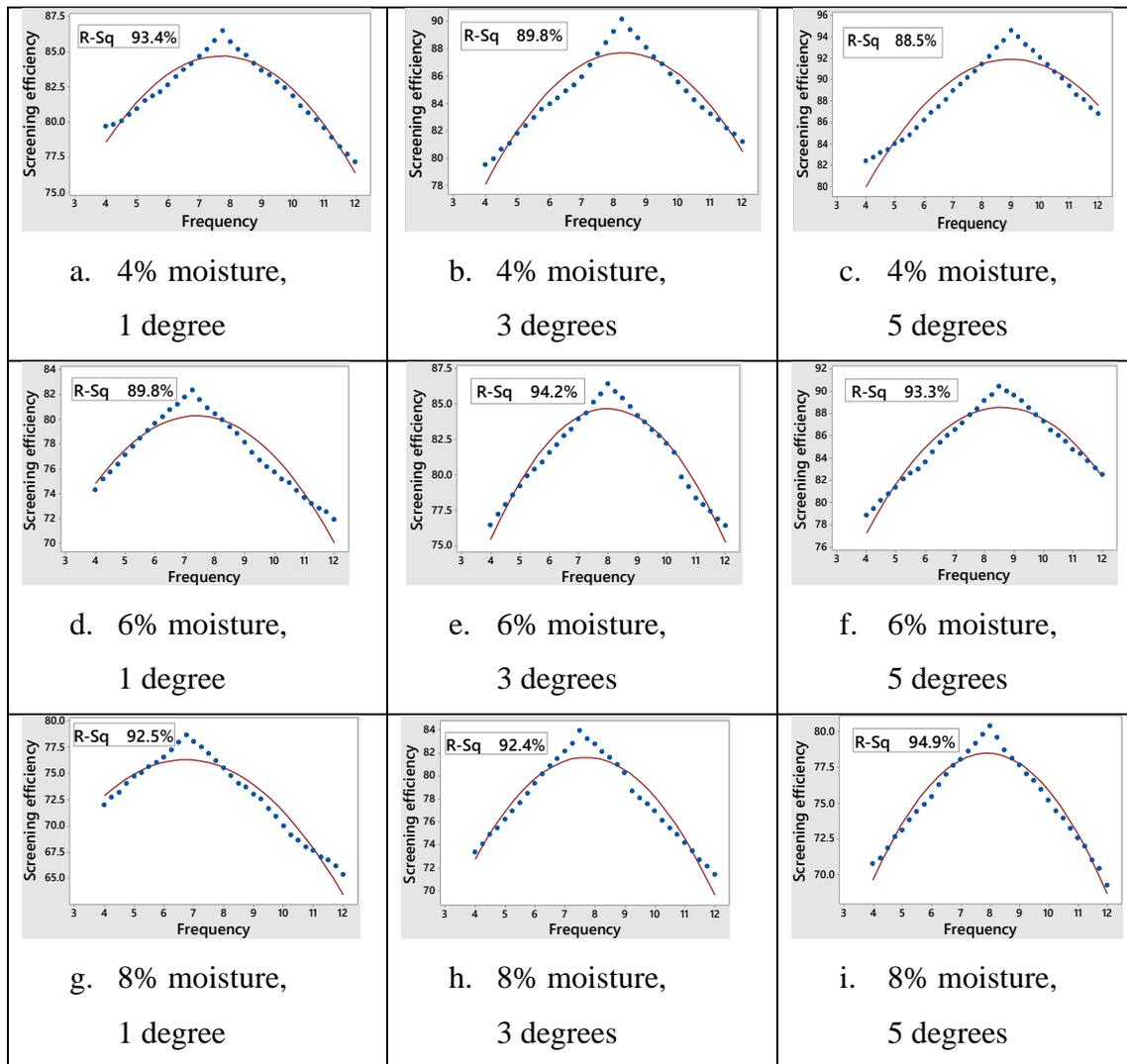
Fig. 4.13 Regression data fitting results for all the conditions of screening iron ore
