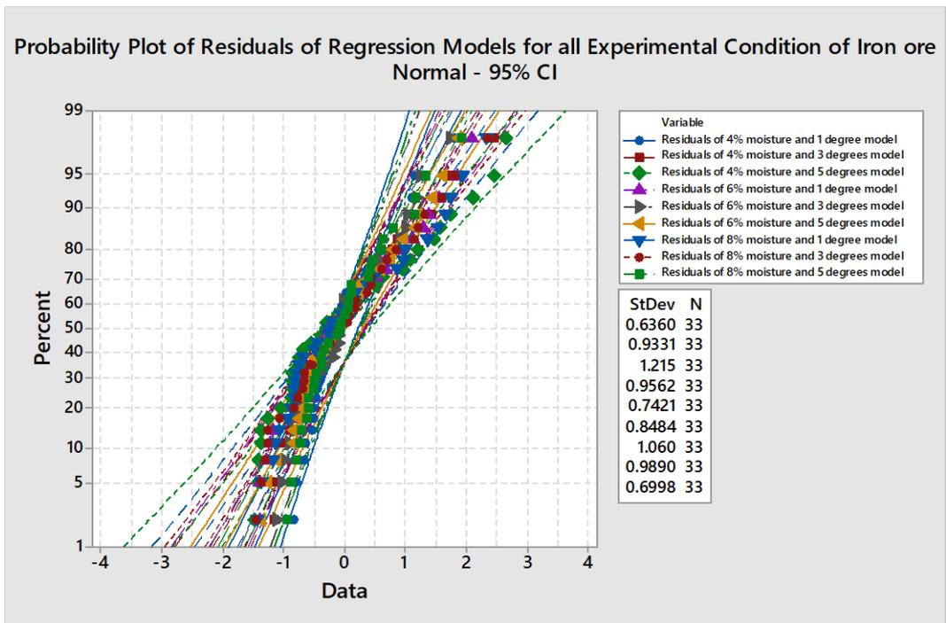
Fig. 4.18 Probability plot of residual of regression models for all the experimental conditions of iron ore
