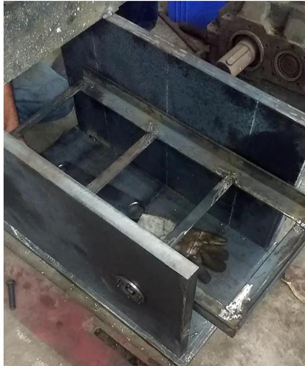
Fig. 3.14 Assembly of the screen deck
