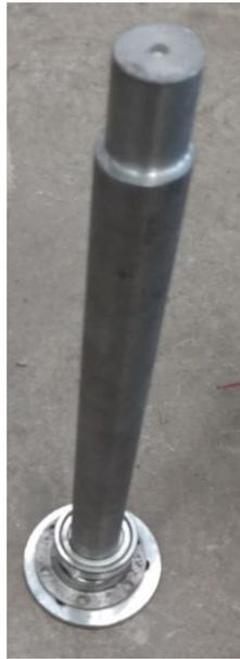
Fig. 3.9 Isometric view and fabricated part of the eccentric shaft
