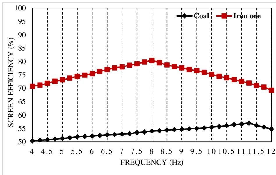
Fig. 4.9 Vibratory screen efficiency of coal and iron ore maintained at 8% moisture and 5°
