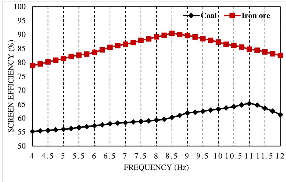
Fig. 4.6 Vibratory screen efficiency of coal and iron ore maintained at 6% moisture and 5°
