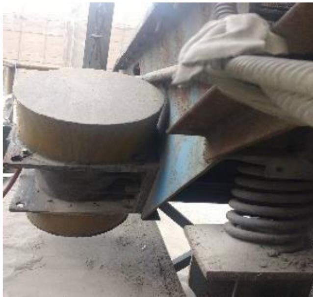
Fig. 3.4 Vibrating motor in the conventional vibrating screen
