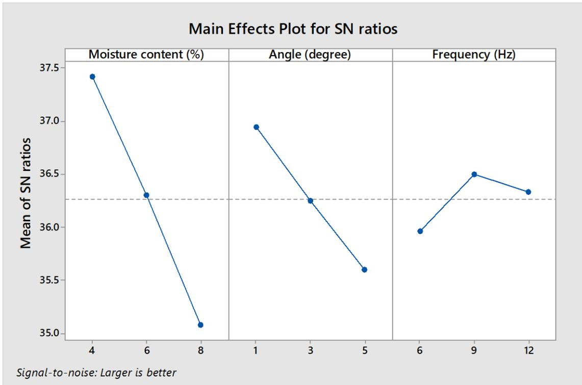
Fig. 4.24 Main effect plot obtained for moisture content, angle, and frequency on coal screening performance
