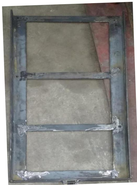
Fig. 3.7 Isometric view and fabricated part of the screen deck
