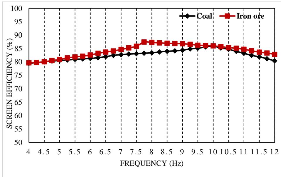
Fig. 4.1 Vibratory screen efficiency of coal and iron ore maintained at 4% moisture and 1<sup>0</sup>
