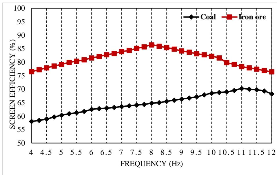
Fig. 4.5 Vibratory screen efficiency of coal and iron ore maintained at 6% moisture and 3°
