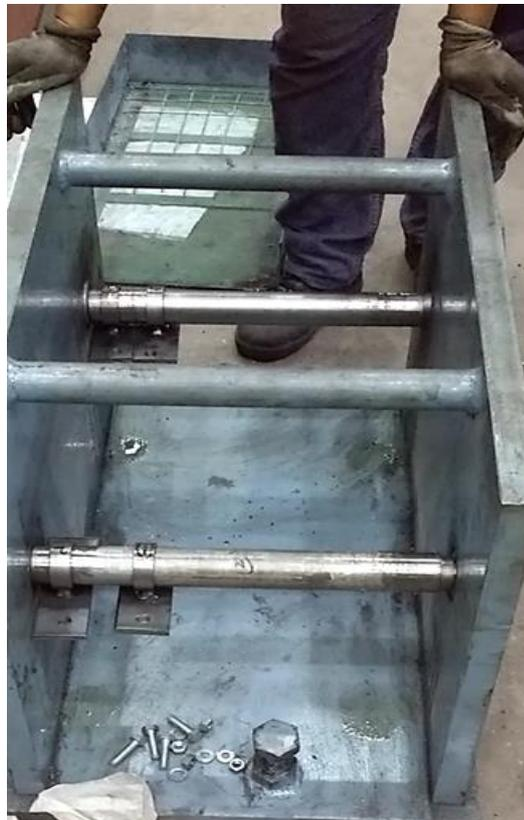
Fig. 3.13 Assembly of the screen holder on the shafts
