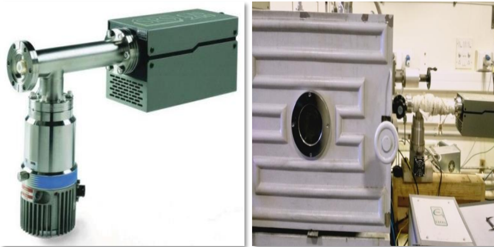
Figure 2.6: (a) SRS 200 RGA with differential pumping mechanism, (b) RGA integration with the process chamber
