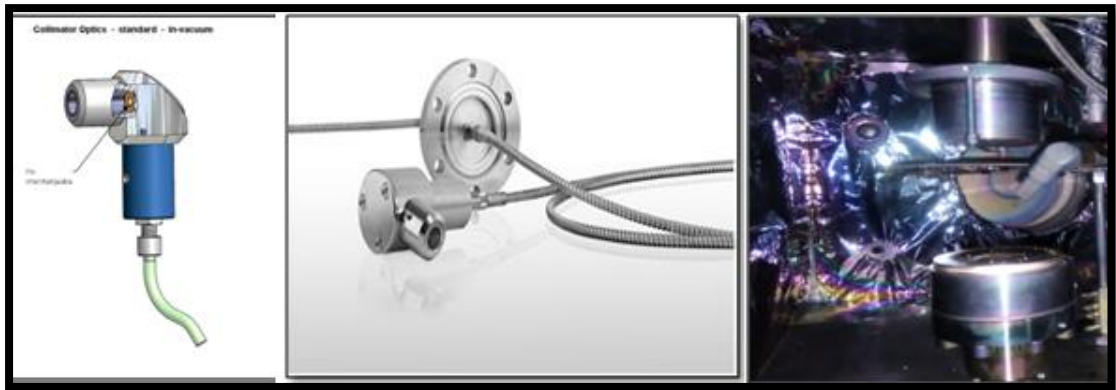
Figure 2.9: Optical emission spectrometer and its incorporation with the process chamber between the magnetron gun and the substrate holder
