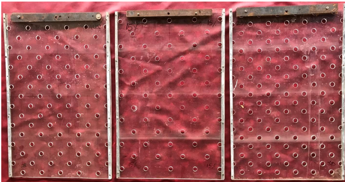
Figure 3.9 Photographic of porous baffles (a) 6.8%, (b) 4.4% and, (c) 9.2%
