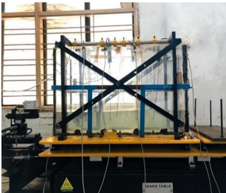
Figure 3.5 Experimental setup of shake table with liquid sloshing tank
