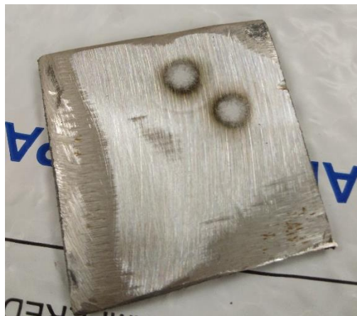
Figure 3.2: Tested specimen for Spectrometric analysis of material
