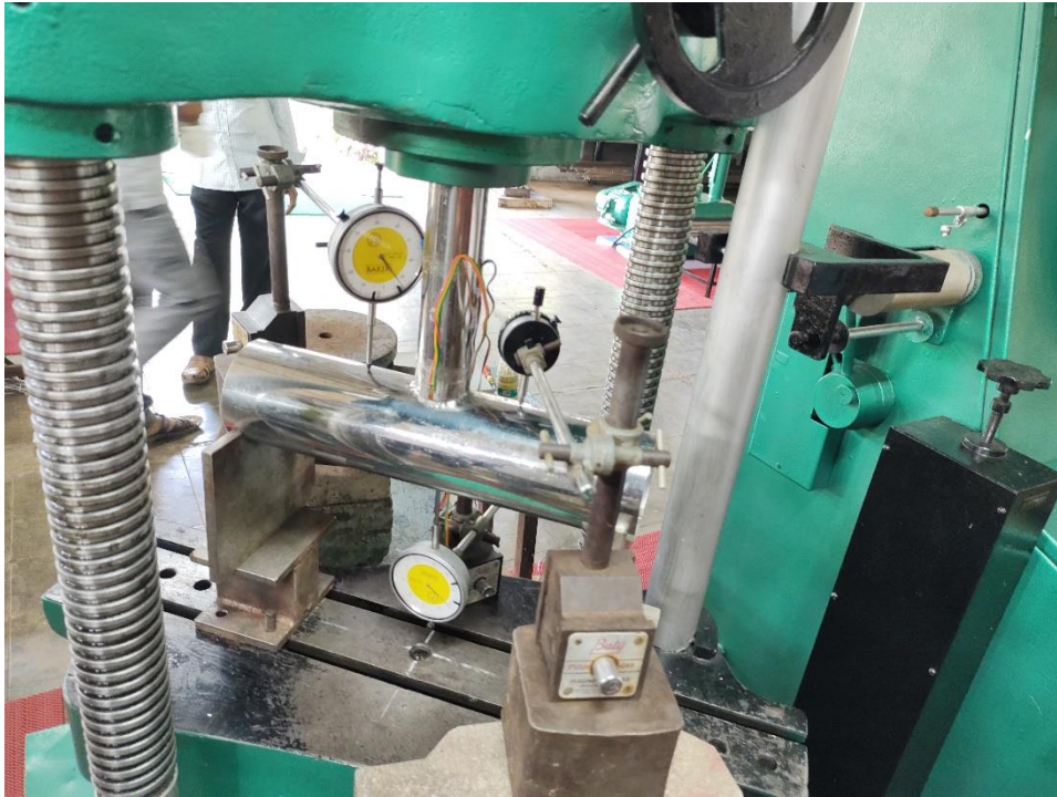
Figure 3.18: Experimental setup with specimen (Unreinforced)
