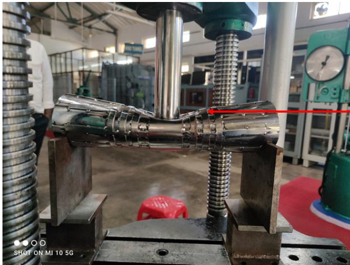
(a) Local collapse of chord wall
