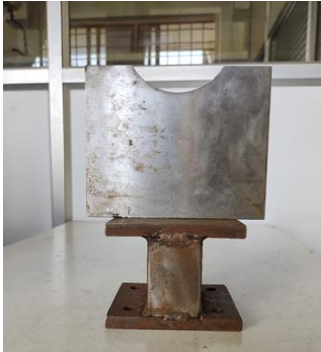
Figure 3.16c: Fabricated saddle support
